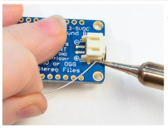
Place the JST and solder that pad onto the connector to tack it in place
