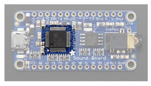
This big chip is the audio decoding engine. It has OGG and WAV decoding capability and can listen to the trigger pins to know when to play each file. It has great audio quality, much better than trying to have a microcontroller generate the audio on its own.
