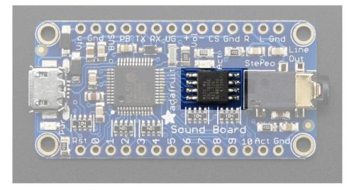
This is the onboard flash chip. It's basically like a little SD card, but soldered directly onto the PCB. These chips can store a few megabytes. This doesn't seem like much but for most audio effects, you don't need hours of music. You can store a couple minute's worth of compressed OGG on a 2M flash chip.
