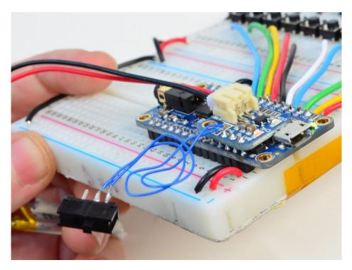
The Lipoly backpack lets you plug in a lipoly battery of any size and recharge it over the MicroUSB connector, so it's basically an all-in-one portable + rechargable system.
