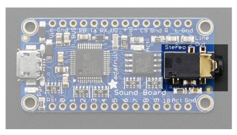
All the way to the right is the headphone jack. This is for connecting to a pair of headphones or into a powered speaker. It cannot drive an 8 ohm or 4 ohm speaker. Instead, an amplifier will have to be used (basically, just like your phone or pocket MP3 player needs an external powered/amplified speaker)
