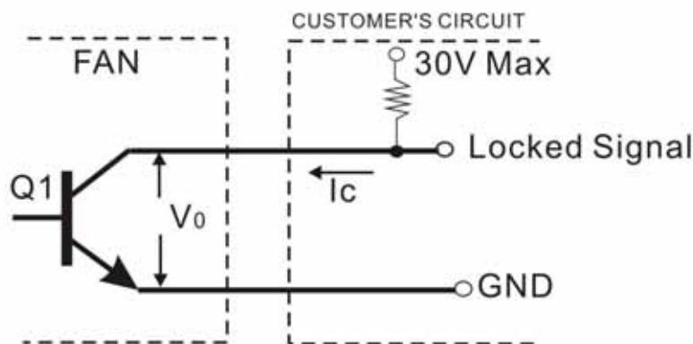
\*Transistor Q1 at "ON" position
