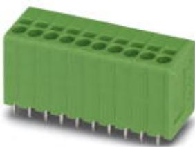
PCB terminal block, Nominal current: 17.5 A, Nom. voltage: 200 V, Pitch: 3.5 mm, Number of positions: 7, Connection method: Push-in spring connection, Mounting: Wave soldering, Conductor/PCB connection direction: 90 °, Color: green
