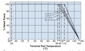
For resistors operated terminal part temperature of described for each size or above, a power rating shall be derated in accordance with derating curve. Please refer to "Introduction of the derating curves based on the terminal part temperature" in the beginning of our catalog before use.
