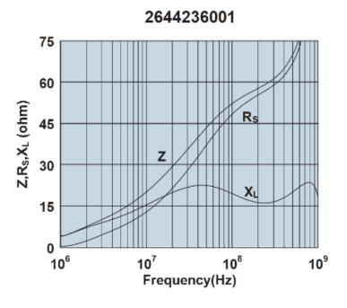
Impedance, reactance, and resistance vs. frequency.
