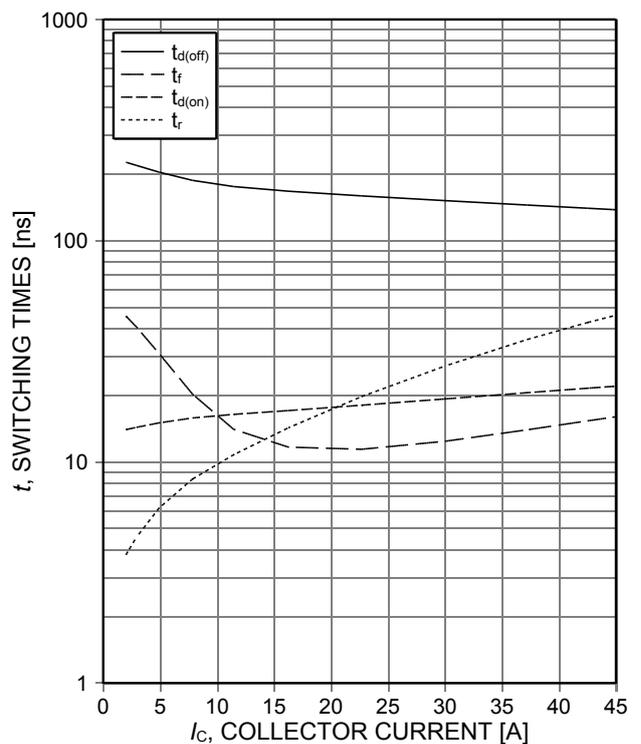
Figure 8. Typical switching times as a function of collector current (inductive load,  $T_{vj}=150^{\circ}\text{C}$ ,  $V_{CE}=400\text{V}$ ,  $V_{GE}=15/0\text{V}$ ,  $r_G=39\Omega$ , Dynamic test circuit in Figure E)
