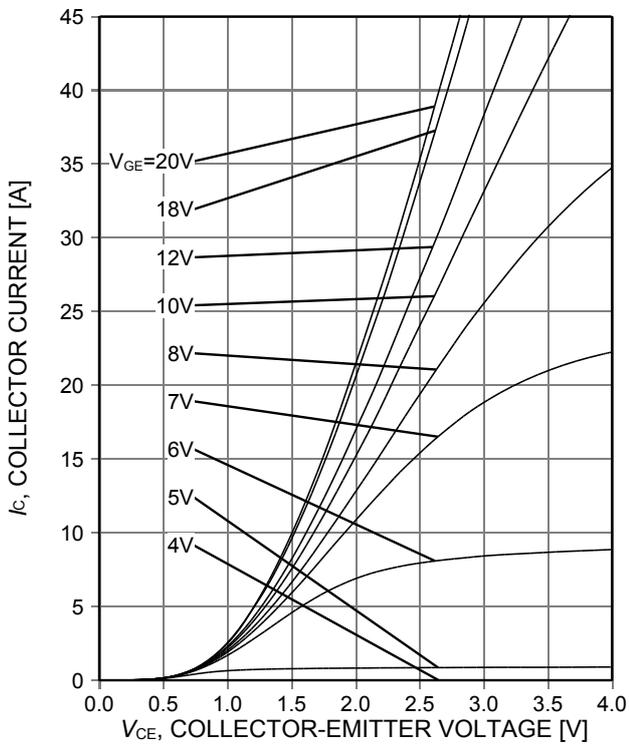
Figure 5. Typical output characteristic ( $T_{vj}=150^{\circ}\text{C}$ )
