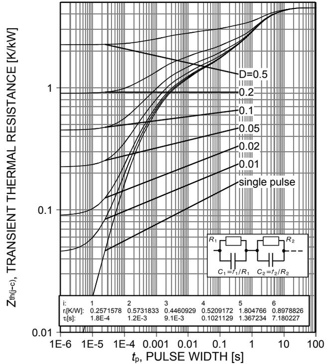
Figure 18. IGBT transient thermal resistance ( $D=t_p/T$ )
