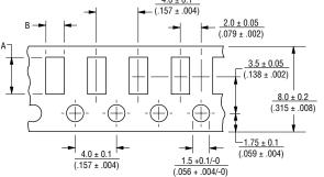
Maximum 1 mm (.040) thick \*Cumulative tolerance over 10 holes: ±0.2 mm
