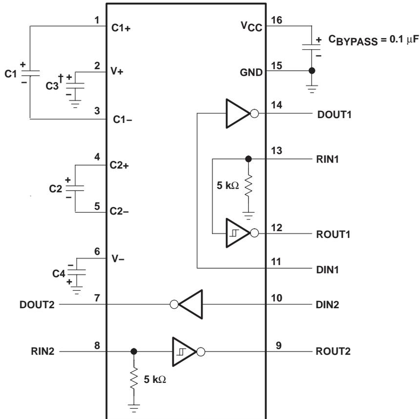
† C3 can be connected to V<sub>CC</sub> or GND.
