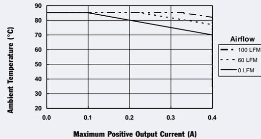
**Note A:** Characteristic data has been developed from actual products tested at 25°C. This data is considered typical data for the Converter.
