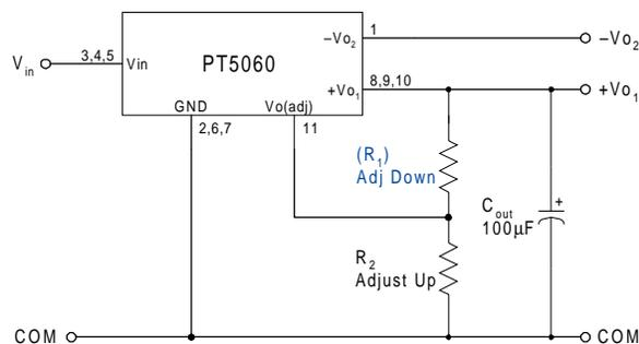
The values of ( $R_1$ ) [adjust down], and  $R_2$  [adjust up], can also be calculated using the following formulas.
