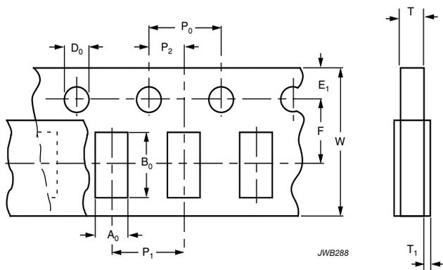
**DIMENSIONS OF PAPER TAPE** in millimeters
