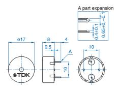
Tolerance: ±0.3 Dimensions in mm
