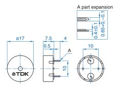
Tolerance: ±0.3 Dimensions in mm
