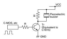
$<sup>^*</sup>$  Resistor to do charging and discharging to a piezoelectric element (Value of about 1k $\!\Omega$  is good efficiency).
