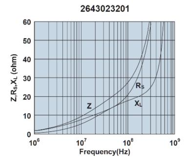
Impedance, reactance, and resistance vs. frequency.
