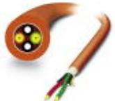
rugged GOF installation cable (IP20 heads only) for inner areas with highly tear-proof aramid strain-relief elements. Individual elements consist of highly flexible FRNC material. The cable is halogen-free, ozone and UV resistant and has a rugged polyurethane (PUR) outer sheath.
