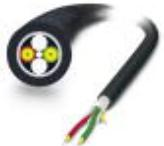
Highly rugged GOF round cable (IP20 heads only) for assembly and for outdoor installation with integrated moisture barrier as well as rodent-proof scrim. Individual elements made from highly flexible FRNC material. The wire is ozone and UV resistant with a very rugged polyethylene outer sheath.
