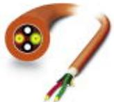
rugged GOF installation cable for inner areas with highly tear-proof aramid strain-relief elements. Individual elements consist of highly flexible FRNC material. The cable is halogen-free, ozone and UV resistant and has a rugged polyurethane (PUR) outer sheath.
