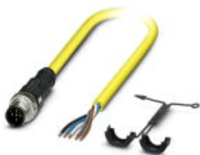
Sensor/actuator cable, 5-position, PVC, yellow, Plug straight M12 SPEEDCON, A-coded, on free cable end, cable length: 2 m
