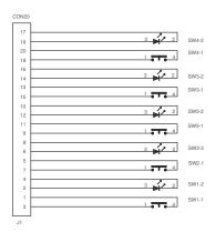
The connector on the illuminated Navimed module is CI1120M1H or similar. We recommend using: Cable socket: Cvilux Cl1120S0000 or similar
