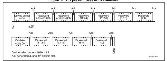
Figure 12. I<sup>2</sup>C present password command
