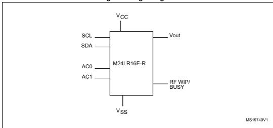
Figure 1. Logic diagram
