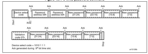
Figure 13. I<sup>2</sup>C write password command
