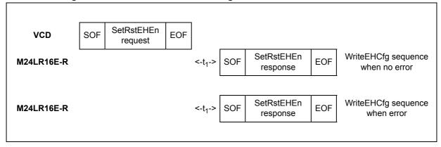
When configured in the RF busy mode, the RF WIP/BUSY pin is tied to 0 from the SOF that starts the SetRstEHEn command to the end of the M24LR16E-R response.
