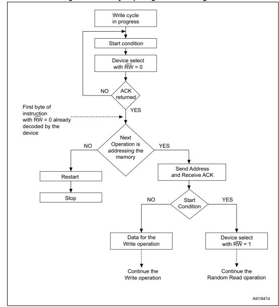
Figure 10. Write cycle polling flowchart using ACK
