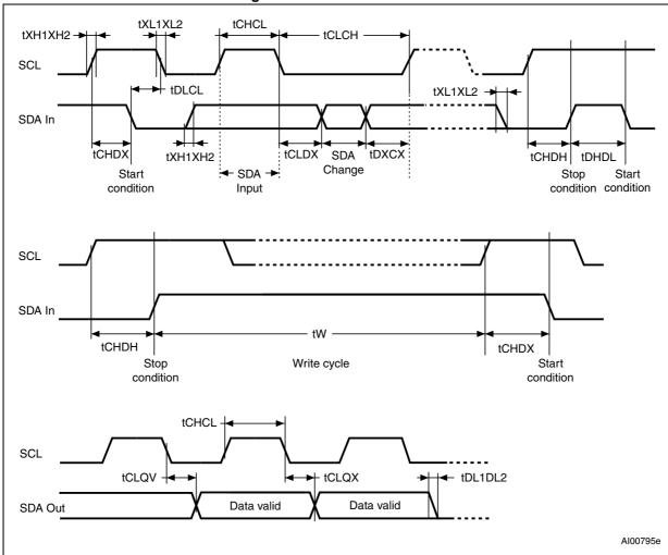
Figure 81. I<sup>2</sup>C AC waveforms
