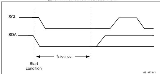
Figure 7. I<sup>2</sup>C timeout on Start condition
