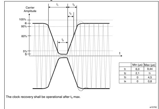
Figure 14. 100% modulation waveform
