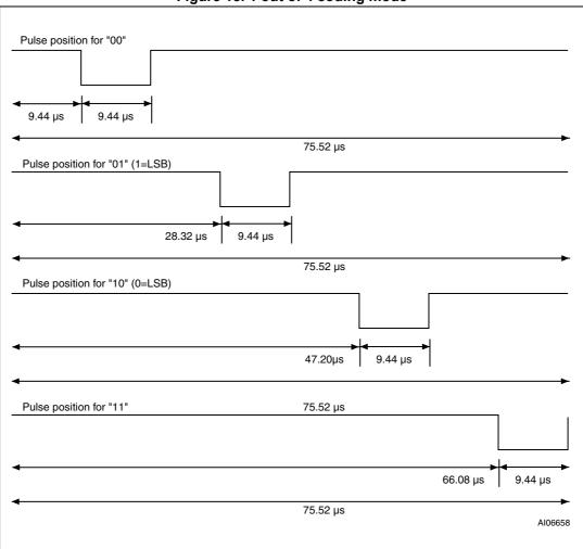
Figure 18. 1 out of 4 coding mode
