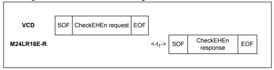
When configured in the RF busy mode, the RF WIP/BUSY pin is tied to 0 from the SOF that starts the CheckEHEn command to the end of the M24LR16E-R response.
