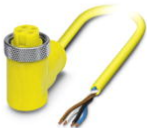
Sensor/actuator cable, 4-position, PVC, yellow, free cable end, on Socket angled 7/8"-16UNF, A-coded, cable length: 4 m
