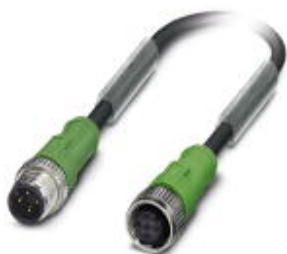
Sensor/actuator cable, 4-position, Special TPE halogen-free, highly flexible, gray RAL 7001, Plug straight M12, A-coded, on Socket straight M12, A-coded, cable length: 10 m
