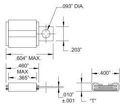
"T" (thickness) depending on capacitance value= .110 to .165±.015
