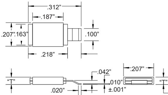
"T" (thickness) depending on capacitance value = .065 to .125±.015
