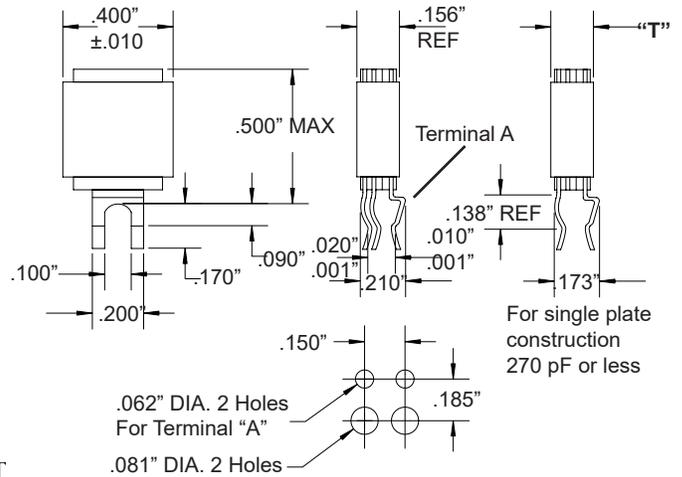
"T" (thickness) depending on capacitance value = .110 to .165±.015
