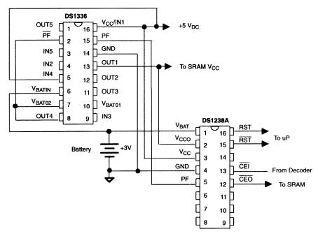
Note: If freshness on the DS1238A is not used,  $\overline{PF}$  on the DS1336 may be tied to OUT1. This will free IN4, OUT4, and  $V_{BAT01}$  for system use.
