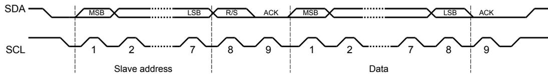
The first seven bits of the first byte make up the slave address (see Figure 13-5 on page 442). The eighth bit determines the direction of the message. A zero in the R/S position of the first byte means that the master will write (send) data to the selected slave, and a one in this position means that the master will receive data from the slave.
