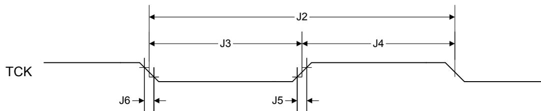
Figure 18-3. JTAG Test Access Port (TAP) Timing
