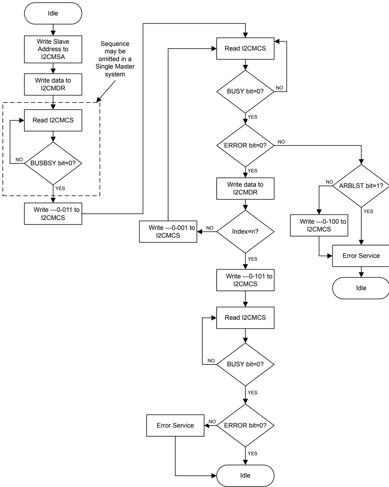
Figure 13-10. Master Burst RECEIVE
