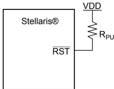
$R_{\text{PU}} = 0$  to 100 k $\Omega$
