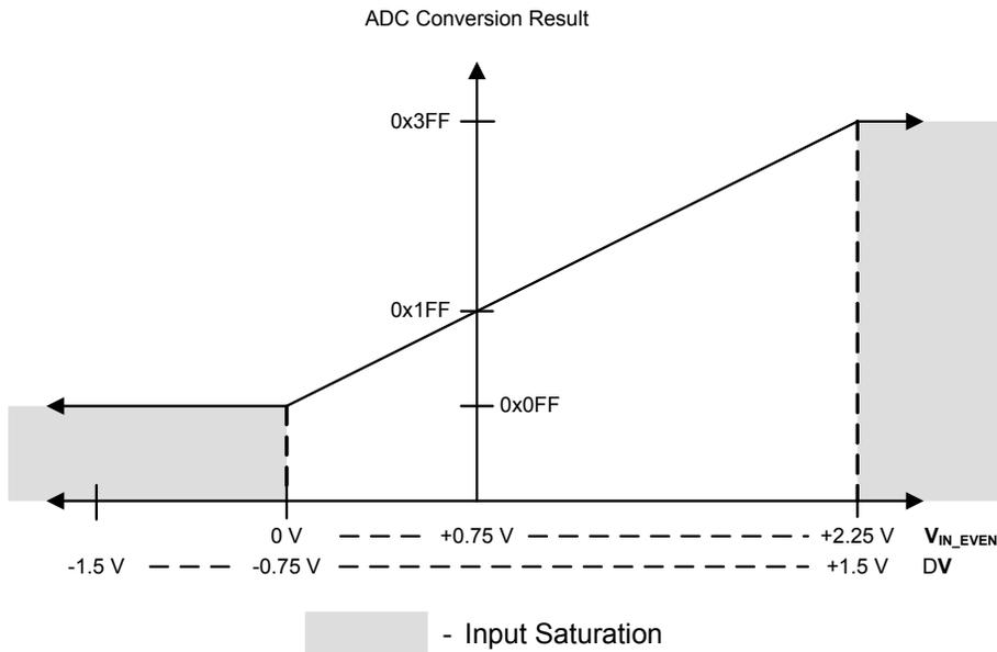
Figure 10-4. Differential Sampling Range,  $V_{IN\_ODD} = 2.25\text{ V}$
