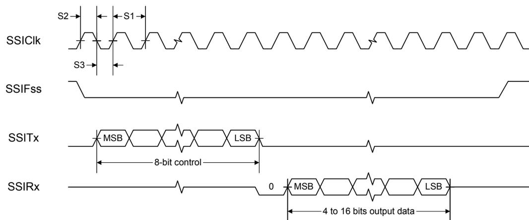
Figure 18-14. SSI Timing for SPI Frame Format (FRF=00), with SPH=1
