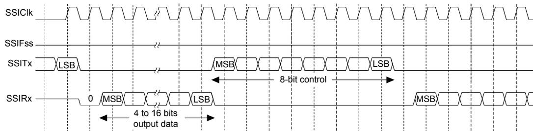
In the MICROWIRE mode, the SSI slave samples the first bit of receive data on the rising edge of SSIClk after SSIFss has gone Low. Masters that drive a free-running SSIClk must ensure that the SSIFss signal has sufficient setup and hold margins with respect to the rising edge of SSIClk.
