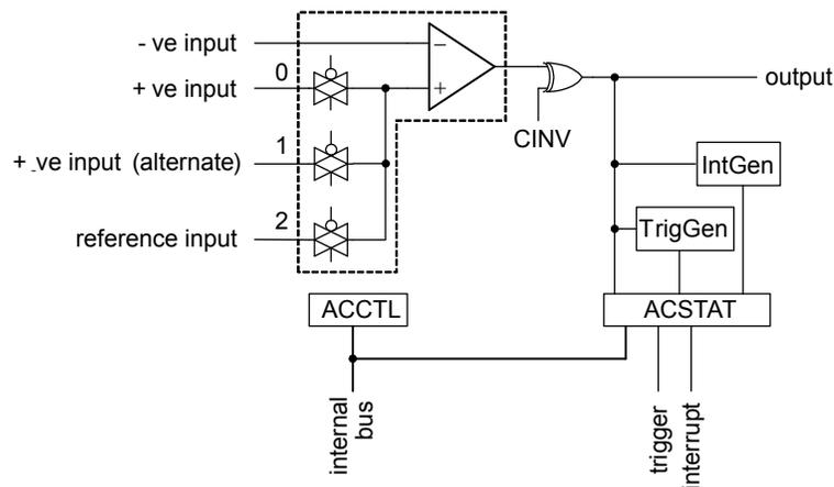
A comparator is configured through two status/control registers (**ACCTL** and **ACSTAT**). The internal reference is configured through one control register (**ACREFCTL**). Interrupt status and control is configured through three registers (**ACMIS**, **ACRIS**, and **ACINTEN**). The operating modes of the comparators are shown in the Comparator Operating Mode tables.
