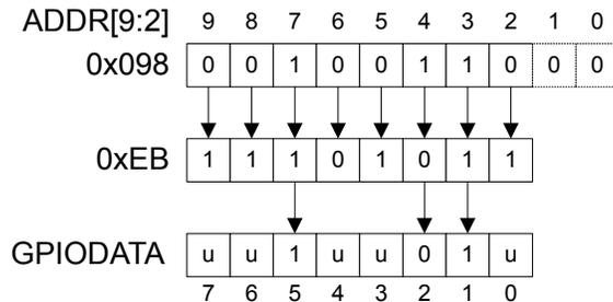
During a read, if the address bit associated with the data bit is set to 1, the value is read. If the address bit associated with the data bit is set to 0, it is read as a zero, regardless of its actual value. For example, reading address **GPIODATA** + 0x0C4 yields as shown in Figure 7-3 on page 229.
