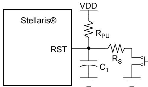
Typical  $R_{PU} = 10 \text{ k}\Omega$
