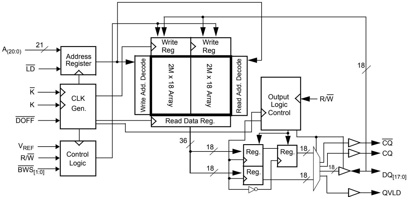
Logic Block Diagram – CY7C1570KV18
