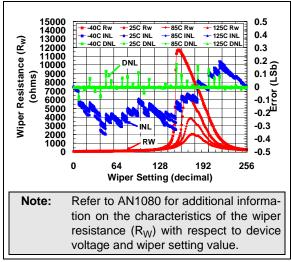
**FIGURE 2-34:** 50 k $\Omega$  Pot Mode –  $R_W(\Omega)$ , INL (LSb), DNL (LSb) vs. Wiper Setting and Ambient Temperature (V<sub>DD</sub> = 1.8V).
