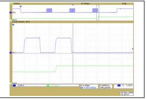
**FIGURE 2-31:** 10 k $\Omega$  – Low-Voltage Increment Wiper Settling Time (V<sub>DD</sub> = 2.7V) (1  $\mu$ s/Div).
