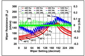
**FIGURE 2-7:** 5 k $\Omega$  Pot Mode –  $R_W(\Omega)$ , INL (LSb), DNL (LSb) vs. Wiper Setting and Ambient Temperature ( $V_{DD} = 3.0V$ ).
