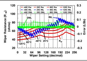
**FIGURE 2-6:**  $5 k\Omega$  Pot Mode  $- R_W(\Omega)$ , INL (LSb), DNL (LSb) vs. Wiper Setting and Ambient Temperature (V<sub>DD</sub> = 5.5V).
