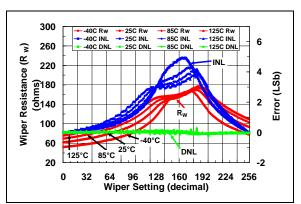
**FIGURE 2-10:** 5 k $\Omega$  Rheo Mode –  $R_W(\Omega)$ , INL (LSb), DNL (LSb) vs. Wiper Setting and Ambient Temperature ( $V_{DD} = 3.0V$ ).
