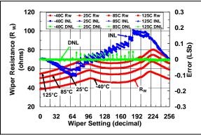
**FIGURE 2-35:** 50 k $\Omega$  Rheo Mode –  $R_W(\Omega)$ , INL (LSb), DNL (LSb) vs. Wiper Setting and Ambient Temperature ( $V_{DD} = 5.5V$ ).
