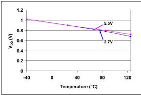
**FIGURE 2-64:** POR/BOR Trip point vs. V<sub>DD</sub> and Temperature.
