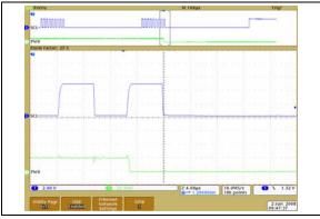
**FIGURE 2-54:** 100 k $\Omega$  – Low-Voltage Decrement Wiper Settling Time (V<sub>DD</sub> = 2.7V) (1  $\mu$ s/Div).
