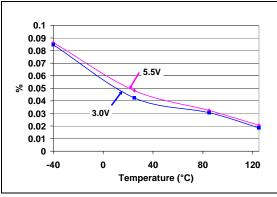
**FIGURE 2-57:** Resistor Network 0 to Resistor Network 1  $R_{AB}$  (5 k $\Omega$ ) Mismatch vs.  $V_{DD}$ and Temperature.
