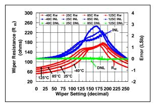
**FIGURE 2-23:** 10 k $\Omega$  Rheo Mode –  $R_W(\Omega)$ , INL (LSb), DNL (LSb) vs. Wiper Setting and Ambient Temperature ( $V_{DD} = 3.0V$ ).
