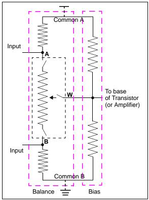
FIGURE 8-3: Example Application Circuit using Terminal Disconnects.
