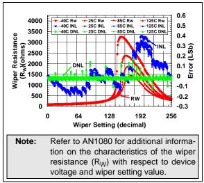
**FIGURE 2-21:** 10 k $\Omega$  Pot Mode –  $R_W(\Omega)$ , INL (LSb), DNL (LSb) vs. Wiper Setting and Ambient Temperature ( $V_{DD} = 1.8V$ ).
