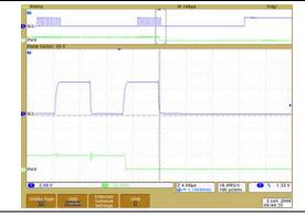
**FIGURE 2-53:** 100 k $\Omega$  – Low-Voltage Decrement Wiper Settling Time (V<sub>DD</sub> = 5.5V) (1  $\mu$ s/Div).
