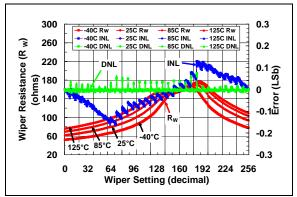
**FIGURE 2-20:** 10 k $\Omega$  Pot Mode –  $R_W(\Omega)$ , INL (LSb), DNL (LSb) vs. Wiper Setting and Ambient Temperature (V<sub>DD</sub> = 3.0V).
