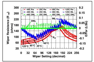
**FIGURE 2-46:** 100 k $\Omega$  Pot Mode –  $R_W(\Omega)$ , INL (LSb), DNL (LSb) vs. Wiper Setting and Ambient Temperature ( $V_{DD} = 3.0V$ ).
