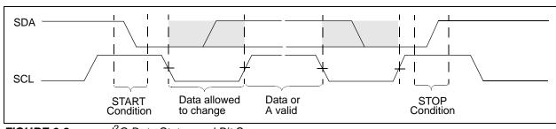
**FIGURE 6-8:** I<sup>2</sup>C Data States and Bit Sequence.
