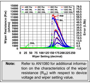
**FIGURE 2-37:** 50 k $\Omega$  Rheo Mode –  $R_W(\Omega)$ , INL (LSb), DNL (LSb) vs. Wiper Setting and Ambient Temperature ( $V_{DD} = 1.8V$ ).
