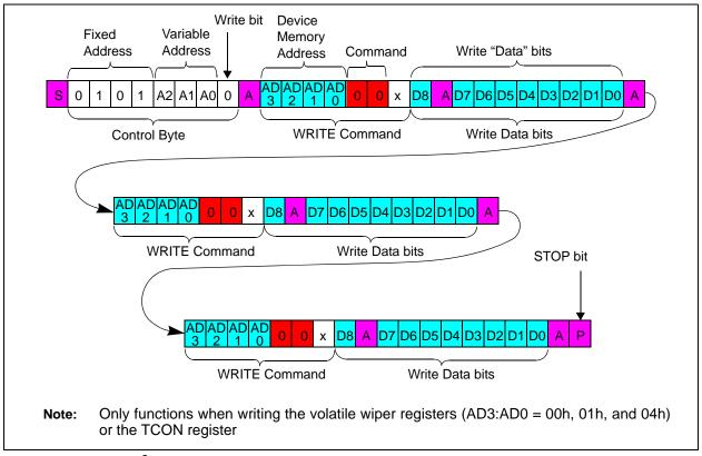
**FIGURE 7-3:** I<sup>2</sup>C Continuous Volatile Wiper Write.
