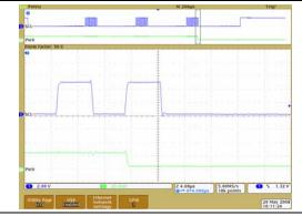
**FIGURE 2-40:** 50 k $\Omega$  – Low-Voltage Decrement Wiper Settling Time (V<sub>DD</sub> = 5.5V) (1  $\mu$ s/Div).
