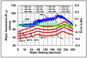
**FIGURE 2-48:** 100 k $\Omega$  Rheo Mode –  $R_W$  ( $\Omega$ ), INL (LSb), DNL (LSb) vs. Wiper Setting and Ambient Temperature ( $V_{DD}$  = 5.5V).
