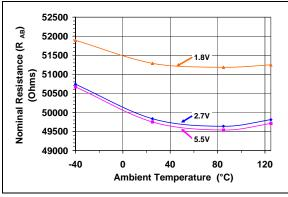
**FIGURE 2-38:** 50 k $\Omega$  – Nominal Resistance ( $\Omega$ ) vs. Ambient Temperature and V<sub>DD</sub>.
