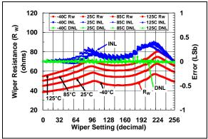
**FIGURE 2-22:** 10 k $\Omega$  Rheo Mode –  $R_W(\Omega)$ , INL (LSb), DNL (LSb) vs. Wiper Setting and Ambient Temperature ( $V_{DD} = 5.5V$ ).
