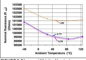
**FIGURE 2-51:** 100 k $\Omega$  – Nominal Resistance ( $\Omega$ ) vs. Ambient Temperature and V<sub>DD</sub>.
