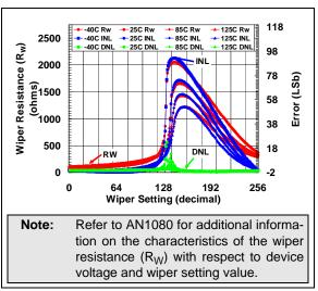
**FIGURE 2-11:** 5 k $\Omega$  Rheo Mode –  $R_W(\Omega)$ , INL (LSb), DNL (LSb) vs. Wiper Setting and Ambient Temperature ( $V_{DD} = 1.8V$ ).
