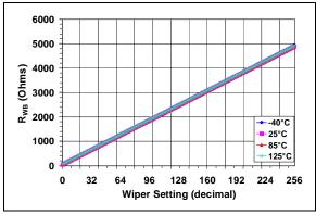
**FIGURE 2-13:**  $5 k\Omega - R_{WB}(\Omega)$  vs. Wiper Setting and Ambient Temperature.
