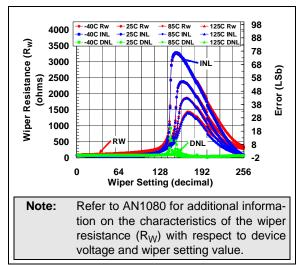
**FIGURE 2-24:** 10 k $\Omega$  Rheo Mode –  $R_W(\Omega)$ , INL (LSb), DNL (LSb) vs. Wiper Setting and Ambient Temperature ( $V_{DD} = 1.8V$ ).
