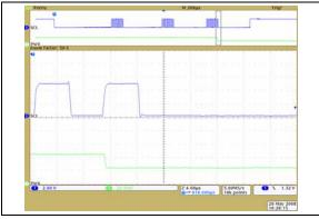
**FIGURE 2-28:** 10 k $\Omega$  – Low-Voltage Decrement Wiper Settling Time (V<sub>DD</sub> = 2.7V) (1  $\mu$ s/Div).
