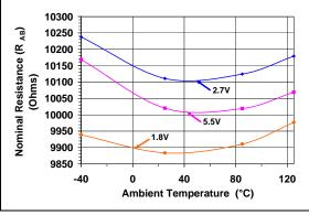
**FIGURE 2-25:** 10 k $\Omega$  – Nominal Resistance ( $\Omega$ ) vs. Ambient Temperature and V<sub>DD</sub>.
