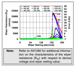
**FIGURE 2-50:** 100 k $\Omega$  Rheo Mode –  $R_W$  ( $\Omega$ ), INL (LSb), DNL (LSb) vs. Wiper Setting and Ambient Temperature ( $V_{DD} = 1.8V$ ).
