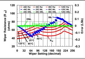
**FIGURE 2-32:** 50 k $\Omega$  Pot Mode –  $R_W(\Omega)$ , INL (LSb), DNL (LSb) vs. Wiper Setting and Ambient Temperature ( $V_{DD} = 5.5V$ ).
