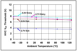
**FIGURE 2-5:** HVC High Input Entry/Exit Threshold vs. Ambient Temperature and V<sub>DD</sub>.
