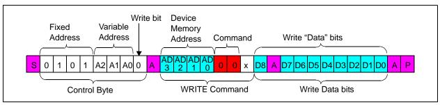
FIGURE 7-2: I<sup>2</sup>C Write Sequence.
