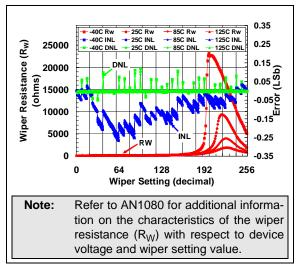
**FIGURE 2-47:** 100 k $\Omega$  Pot Mode –  $R_W(\Omega)$ , INL (LSb), DNL (LSb) vs. Wiper Setting and Ambient Temperature ( $V_{DD} = 1.8V$ ).
