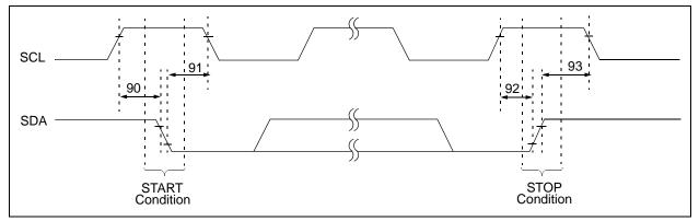
FIGURE 1-1: I<sup>2</sup>C Bus Start/Stop Bits Timing Waveforms.
