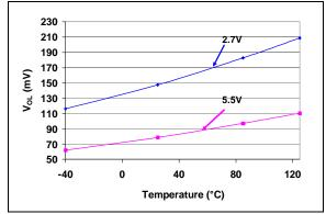
**FIGURE 2-63:**  $V_{OL}$  (SDA) vs.  $V_{DD}$  and Temperature ( $I_{OL} = 3$  mA).
