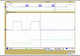
**FIGURE 2-30:** 10 k $\Omega$  – Low-Voltage Increment Wiper Settling Time (V<sub>DD</sub> = 5.5V) (1  $\mu$ s/Div).
