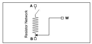
FIGURE 5-2: Resistor Network Shutdown Configuration.
