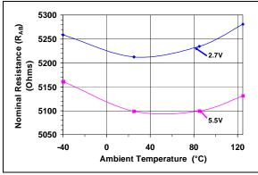
**FIGURE 2-12:**  $5 k\Omega$  – Nominal Resistance ( $\Omega$ ) vs. Ambient Temperature and V<sub>DD</sub>.
