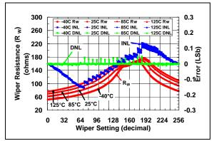
**FIGURE 2-33:** 50 k $\Omega$  Pot Mode –  $R_W(\Omega)$ , INL (LSb), DNL (LSb) vs. Wiper Setting and Ambient Temperature (V<sub>DD</sub> = 3.0V).
