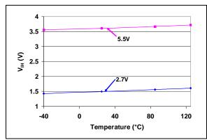
**FIGURE 2-61:** V<sub>IH</sub> (SDA, SCL) vs. V<sub>DD</sub> and Temperature.
