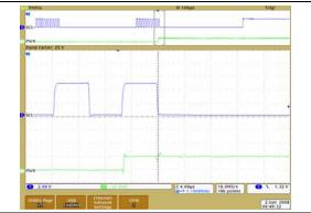
**FIGURE 2-55:** 100 k $\Omega$  – Low-Voltage Increment Wiper Settling Time (V<sub>DD</sub>=5.5V) (1  $\mu$ s/Div).
