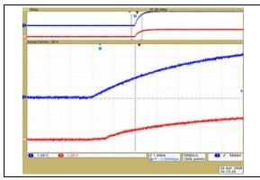
**FIGURE 2-42:** 50 k $\Omega$  – Power-Up Wiper Response Time (1  $\mu$ s/Div).
