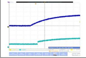
**FIGURE 2-16:**  $5 k\Omega$  – Power-Up Wiper Response Time (20 ms/Div).
