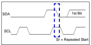
FIGURE 6-5: Repeat Start Condition Waveform.
