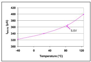
**FIGURE 2-3:** Write Current (I<sub>WRITE</sub>) vs. Ambient Temperature.
