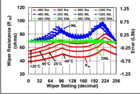
**FIGURE 2-9:** 5 k $\Omega$  Rheo Mode –  $R_W(\Omega)$ , INL (LSb), DNL (LSb) vs. Wiper Setting and Ambient Temperature ( $V_{DD} = 5.5V$ ).
