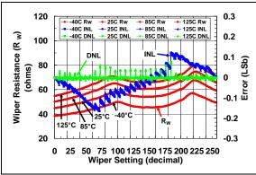
**FIGURE 2-19:** 10 k $\Omega$  Pot Mode –  $R_W(\Omega)$ , INL (LSb), DNL (LSb) vs. Wiper Setting and Ambient Temperature (V<sub>DD</sub> = 5.5V).
