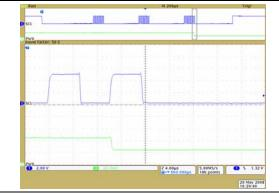
**FIGURE 2-27:** 10 k $\Omega$  – Low-Voltage Decrement Wiper Settling Time (V<sub>DD</sub> = 5.5V) (1  $\mu$ s/Div).
