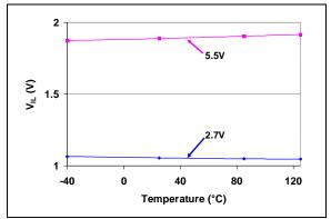
**FIGURE 2-62:**  $V_{IL}$  (SDA, SCL) vs.  $V_{DD}$  and Temperature.
