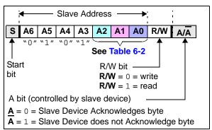
**FIGURE 6-9:** Slave Address Bits in the  $l^2C$  Control Byte.
