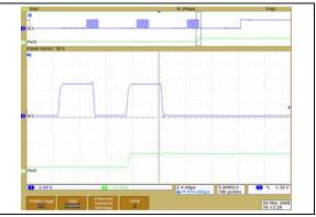
**FIGURE 2-44:** 50 k $\Omega$  – Low-Voltage Increment Wiper Settling Time (V<sub>DD</sub> = 2.7V) (1  $\mu$ s/Div).
