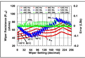
**FIGURE 2-45:** 100 k $\Omega$  Pot Mode –  $R_W(\Omega)$ , INL (LSb), DNL (LSb) vs. Wiper Setting and Ambient Temperature ( $V_{DD} = 5.5V$ ).
