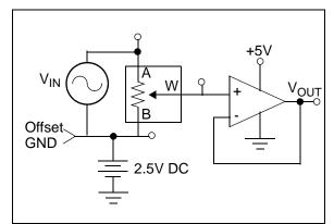
FIGURE 2-65: -3 db Gain vs. Frequency Test.
