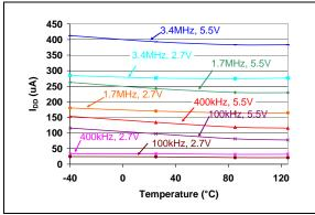
**FIGURE 2-1:** Device Current ( $I_{DD}$ ) vs.  $I^2C$ Frequency ( $f_{SCL}$ ) and Ambient Temperature ( $V_{DD}$  = 2.7V and 5.5V).
