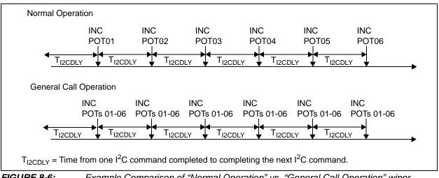
*FIGURE 8-6:* Example Comparison of "Normal Operation" vs. "General Call Operation" wiper Updates.
