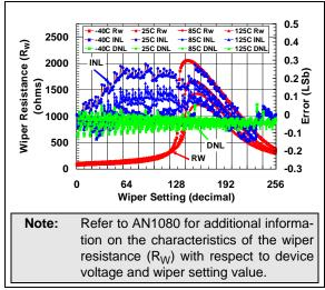
**FIGURE 2-8:** 5 k $\Omega$  Pot Mode –  $R_W(\Omega)$ , INL (LSb), DNL (LSb) vs. Wiper Setting and Ambient Temperature ( $V_{DD} = 1.8V$ ).
