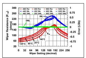
**FIGURE 2-36:** 50 k $\Omega$  Rheo Mode –  $R_W(\Omega)$ , INL (LSb), DNL (LSb) vs. Wiper Setting and Ambient Temperature ( $V_{DD} = 3.0V$ ).
