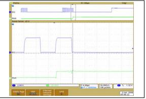
**FIGURE 2-56:** 100 k $\Omega$  – Low-Voltage Increment Wiper Settling Time (V<sub>DD</sub> = 2.7V) (1  $\mu$ s/Div)
