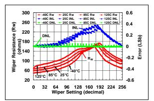
**FIGURE 2-49:** 100 k $\Omega$  Rheo Mode –  $R_W$  ( $\Omega$ ), INL (LSb), DNL (LSb) vs. Wiper Setting and Ambient Temperature ( $V_{DD} = 3.0V$ ).
