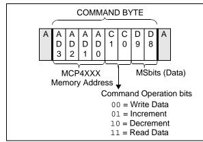
FIGURE 7-1: Command Byte Format.
