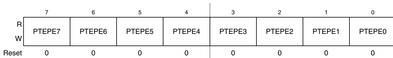
Figure 6-24. Internal Pullup Enable for Port E (PTEPE)
