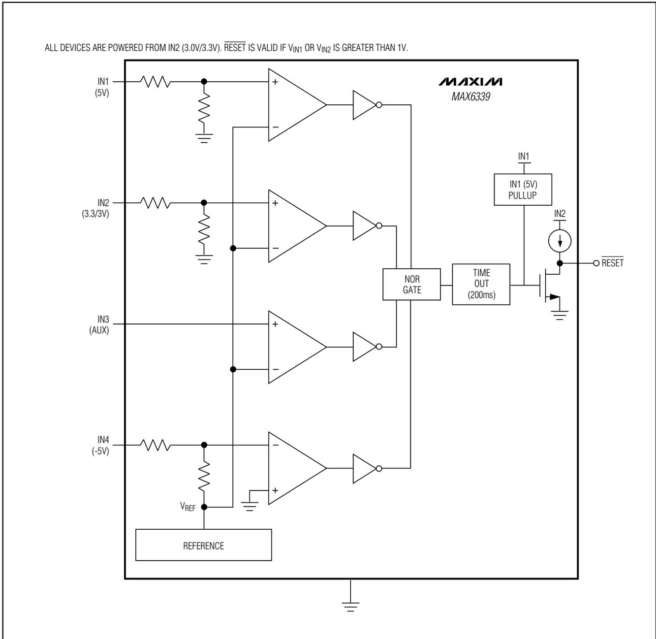
Figure 1. Functional Diagram
