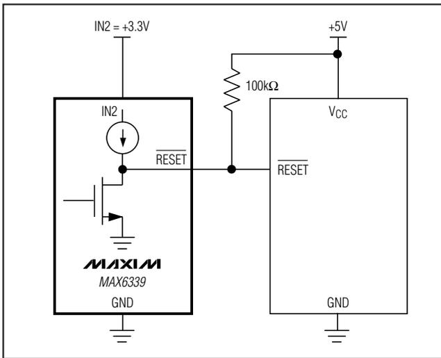
Figure 3. Interfacing to Different Logic Supply Voltage
