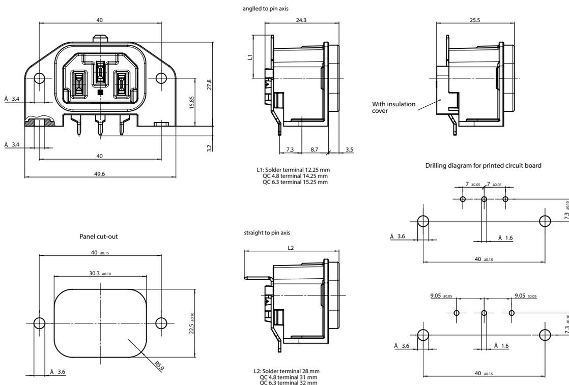
**PIN: Spacing 7 / 9.7mm or 9.05 / 9.7mm**
