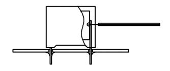
Temperature monitored inside the capacitor.
