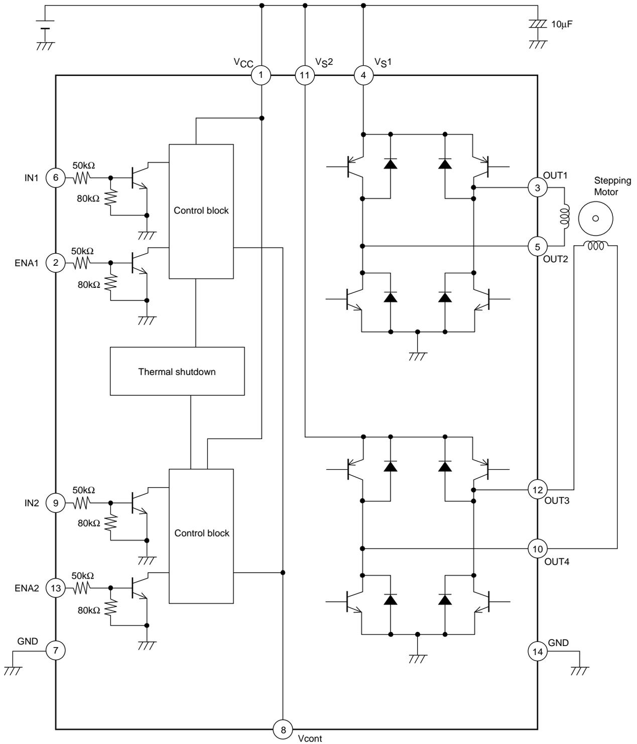
\* There are no constraints on the relationship between the applied voltage to  $V_{CC}$ ,  $V_{S1}$ ,  $V_{S2}$ ,  $EN_{A1}$ ,  $EN_{A2}$ ,  $IN_1$ , and  $IN_2$  within the absolute maximum ratings (For example, this IC can be used at  $V_{CC}=3V$ ,  $V_{S1}=V_{S2}=2V$ , and  $EN_{A1}=EN_{A2}=5V$ )
