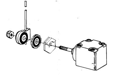
ADJUSTABLE TO OPERATE CLOCKWISE, COUNTER-CLOCKWISE, OR IN BOTH DIRECTIONS.
