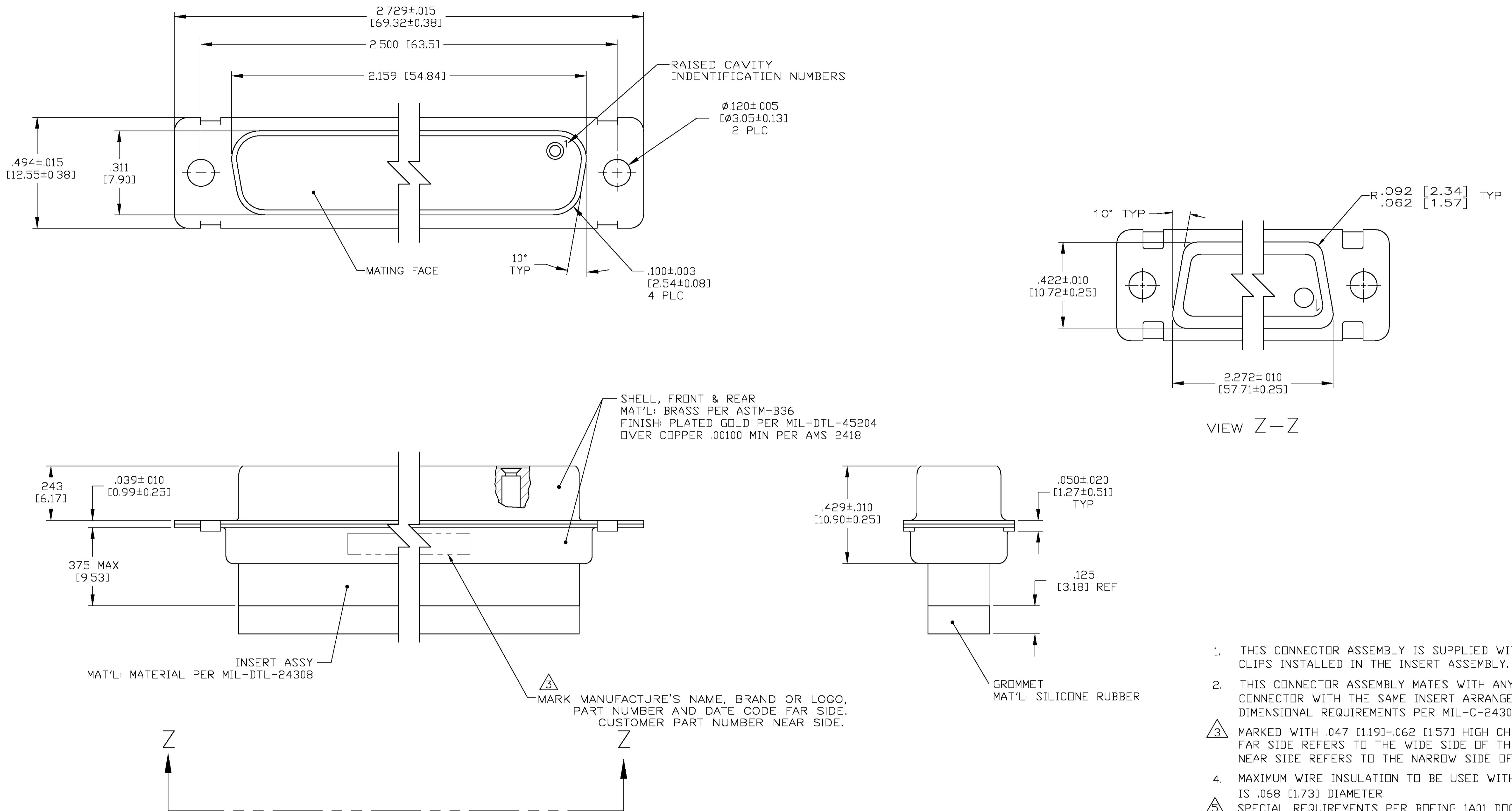
1. THIS CONNECTOR ASSEMBLY IS SUPPLIED WITH Be Cu CONTACT RETENTION CLIPS INSTALLED IN THE INSERT ASSEMBLY.
