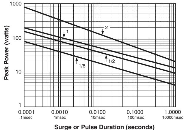
Note: Use for repetitive pulses where the average power dissipation is not to exceed the component rating at 70°C. Surge handling capacity for low-repetitive surges may be significantly greater than shown above. Contact factory for recommendations.
