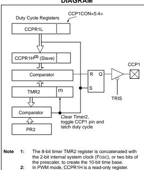
The PWM output (Figure 15-4) has a time base (period) and a time that the output stays high (duty cycle).
