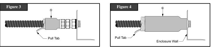
5. Position Cold Shrink Corrosion Protection Assembly (6) (*Figure 4*) over bulkhead termination connector. Install by unwinding loose core pull tab in a counter-clockwise direction around cable. Rubber sleeve should make contact with enclosure wall during installation.
