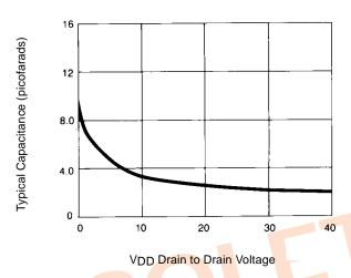
Figure 9. Typical Output Capacitance
