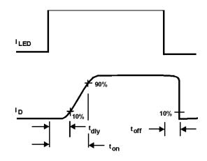
Figure 7. Typical Delay Times
