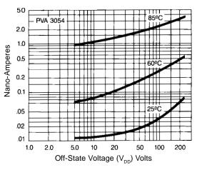
Figure 5. Typical Variation of Off-State Leakage
