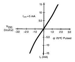
Figure 3.Typical On Characteristics
