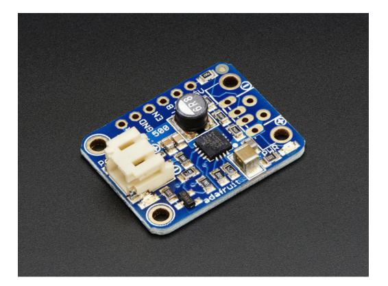
The PowerBoost 500 (https://adafru.it/dFq) has at the heart a TPS61090 boost converter from TI (https://adafru.it/duQ). This boost converter chip has some really nice extras such as low battery detection, 2A internal switch, synchronous conversion, excellent efficiency, and 700KHz high-frequency operation. Check out these specs!
