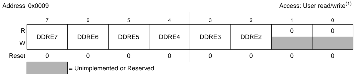
Figure 2-7. Port E Data Direction Register (DDRE)
