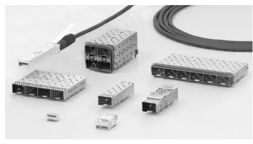
SFP+ extends the use of the Small Form-Factor Pluggable (SFP) interconnect up to 10 Gb/s. This system meets the performance requirements of SFF (Small Form-Factor) specification SFF-8431 and supports 8G Fibre Channel and 10G Ethernet applications. The SFP+ product family includes cages, connectors, and copper cable assemblies. SFP+ cages are offered with both EMI springs and elastomeric
