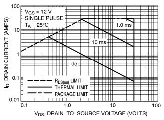
Figure 11. Maximum Rated Forward Biased Safe Operating Area
