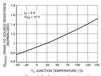
Figure 5. On–Resistance Variation with Temperature
