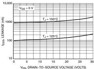
Figure 6. Drain-to-Source Leakage Current versus Voltage
