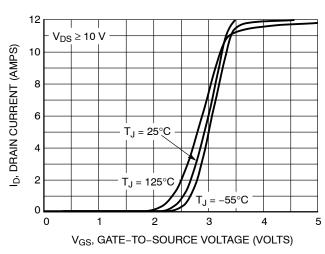
Figure 2. Transfer Characteristics
