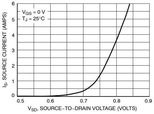
Figure 10. Diode Forward Voltage versus Current
