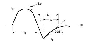
Figure 14. Diode Reverse Recovery Waveform
