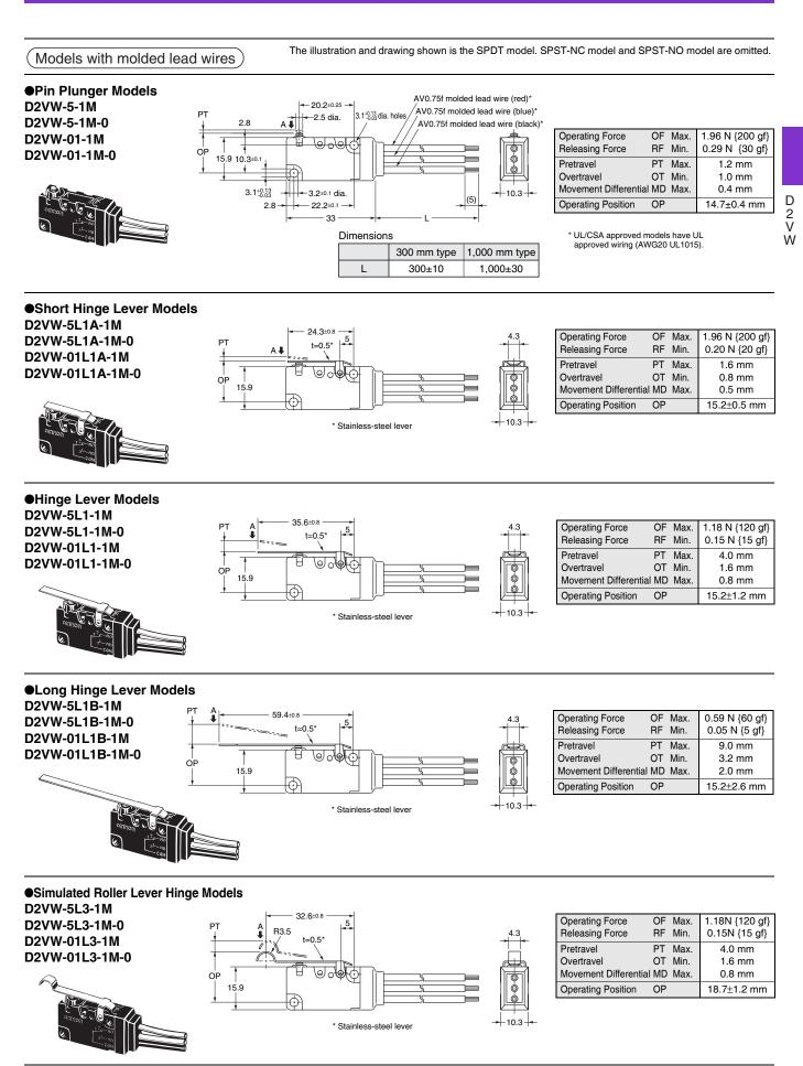
Note 1. Unless otherwise specified, a tolerance of  $\pm 0.4$  mm applies to all dimensions. Note 2. The operating characteristics are for operation in the A direction ( **\**).
