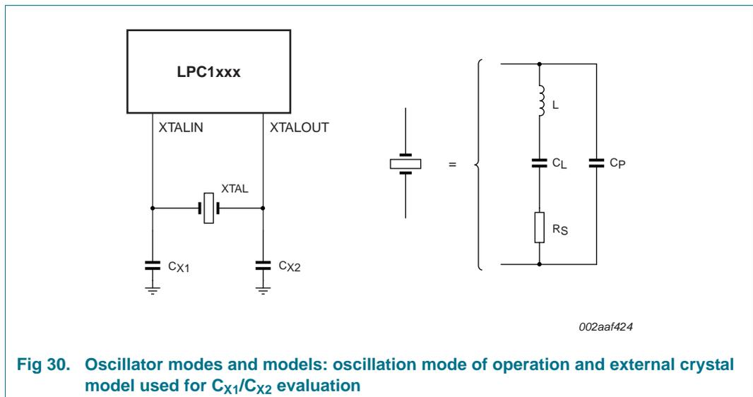
Fig 30. Oscillator modes and models: oscillation mode of operation and external crystal model used for  $C_{X1}/C_{X2}$  evaluation
