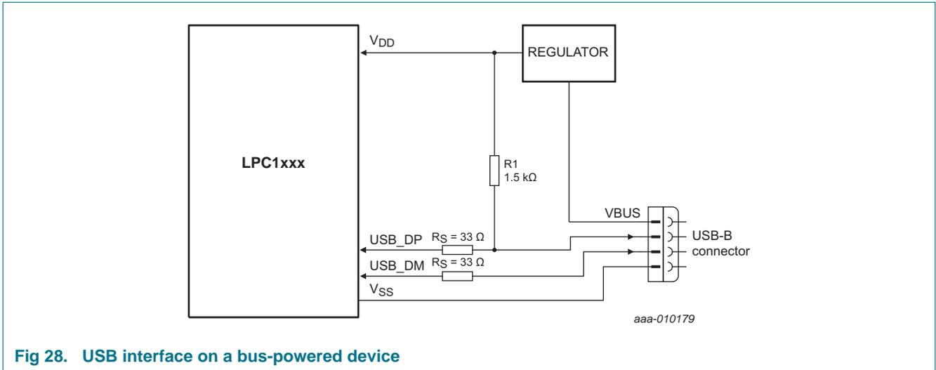
Fig 28. USB interface on a bus-powered device
