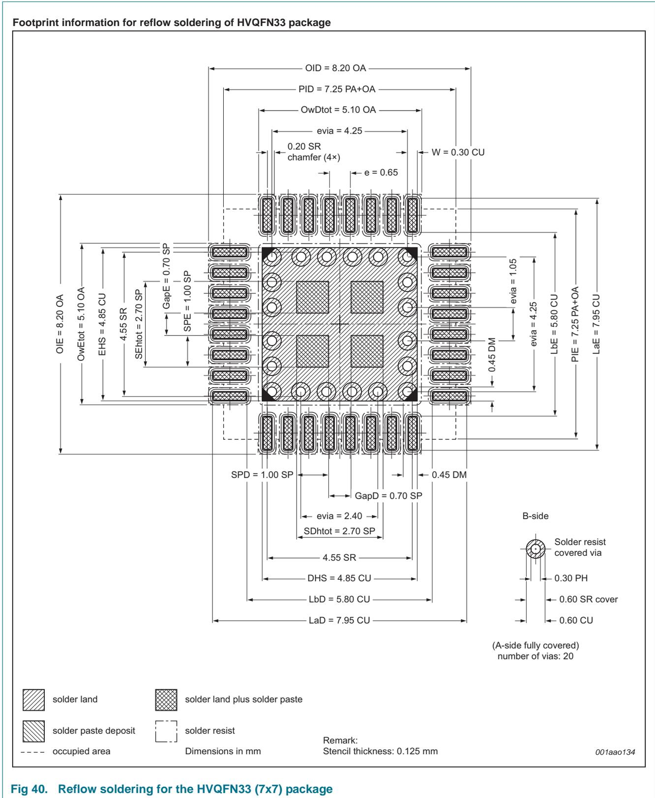
Fig 40. Reflow soldering for the HVQFN33 (7x7) package
