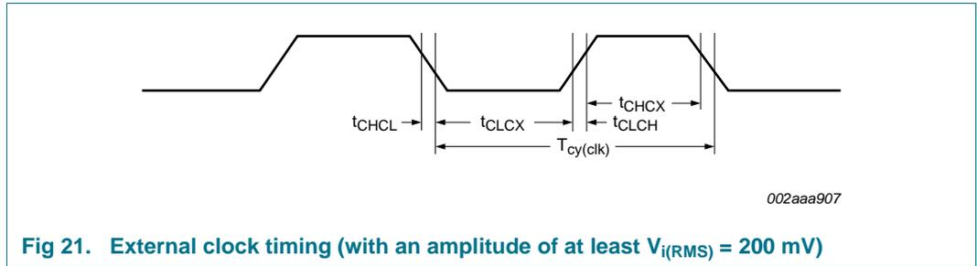
Fig 21. External clock timing (with an amplitude of at least  $V_{i(RMS)} = 200\text{ mV}$ )
