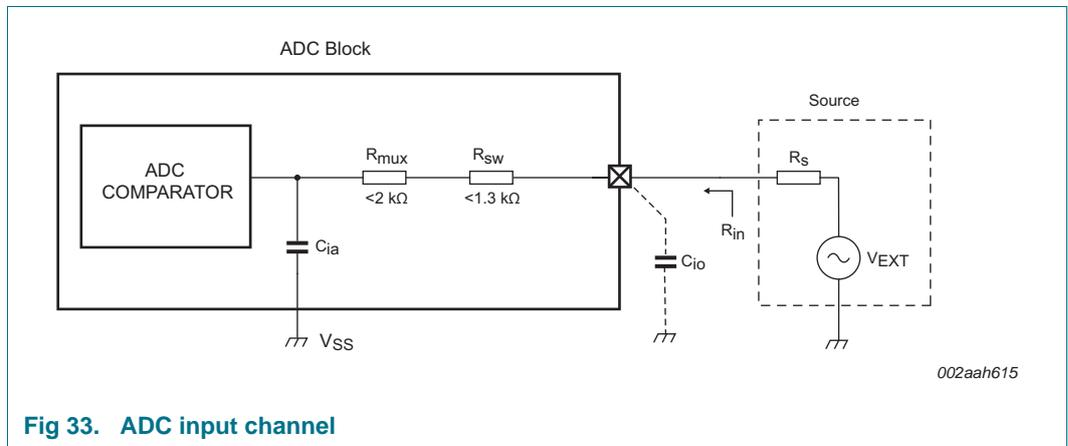
Fig 33. ADC input channel
