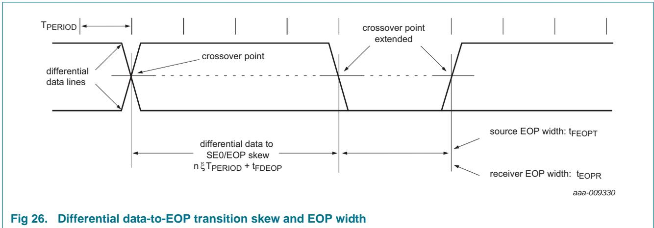
Fig 26. Differential data-to-EOP transition skew and EOP width
