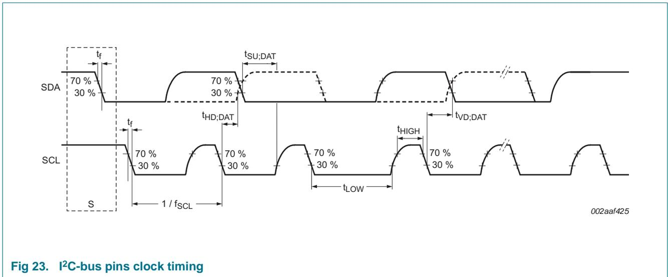
Fig 23. I<sup>2</sup>C-bus pins clock timing
