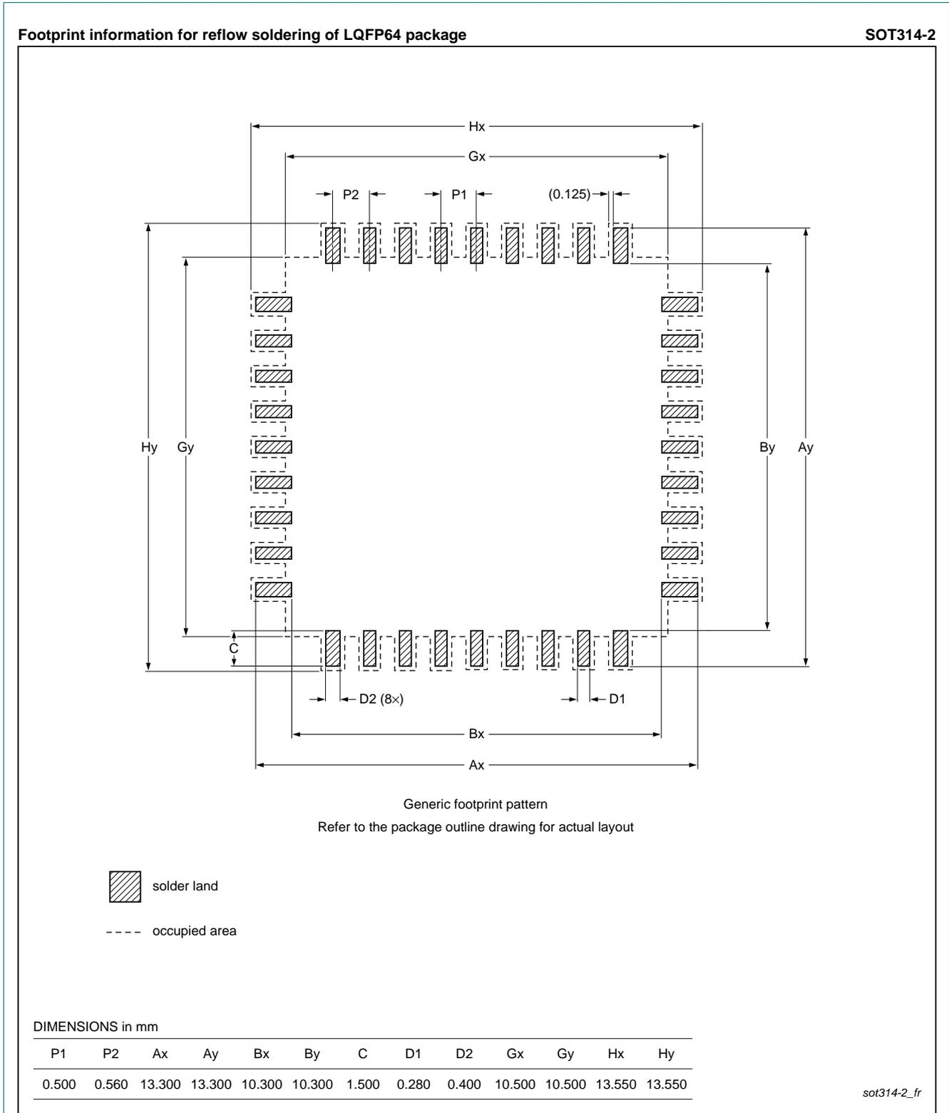
**Fig 43. Reflow soldering for the LQFP64 package**
