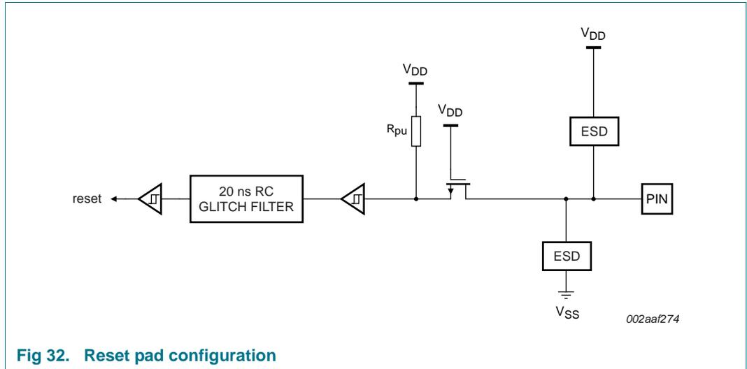
Fig 32. Reset pad configuration
