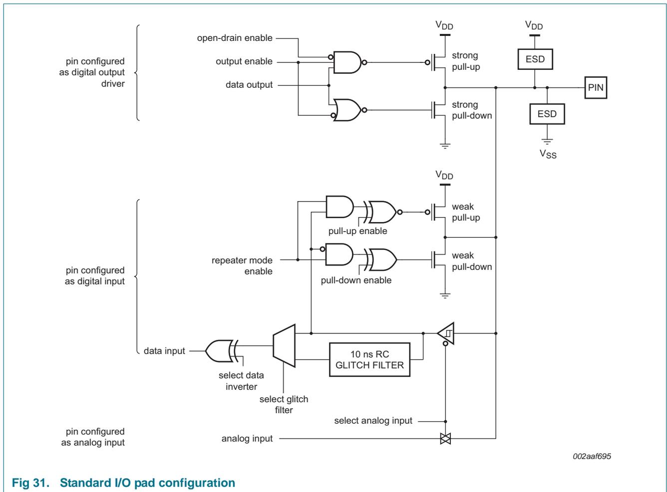
Fig 31. Standard I/O pad configuration
