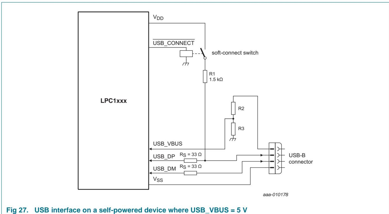
Fig 27. USB interface on a self-powered device where  $USB\_VBUS = 5 \text{ V}$
