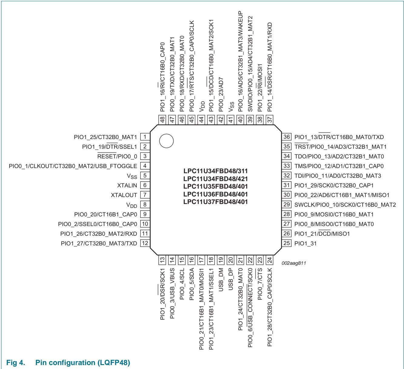
Fig 4. Pin configuration (LQFP48)
