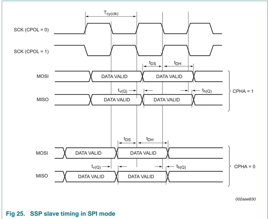
Fig 25. SSP slave timing in SPI mode
