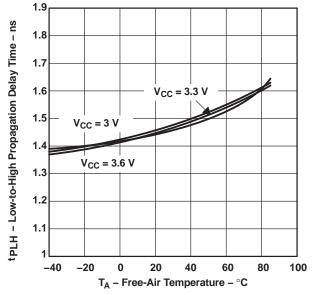
Figure 2. Low-to-High Propagation Delay Time vs Free-Air Temperature
