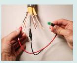
GREEN LED means wiring is properly identified.
