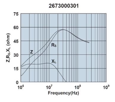
Impedance, reactance, and resistance vs. frequency.
