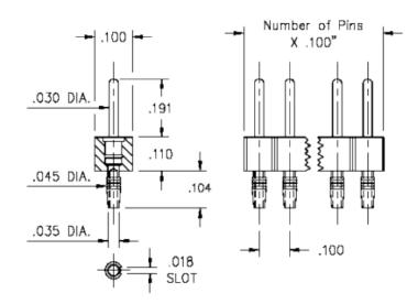
**Description:** Interconnect Header Solderless Press-Fit Pin Header .030" (0,76mm) Pin Head Single Row Through Hole Plating Code: 10 Shell Plating: 10 µ" Gold over 100 µ" Nickel
