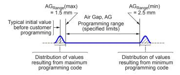
Figure 3. On the horizontal axis, the operating air gap may exceed the recommended range for switching. The maximum and minimum values for the actual operating air gap range are described by distributions of the maximum and minimum code setpoints.
