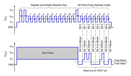
Figure 11. Read mode example. Pulse sequence for accessing the  $B_{OP}$  Selection register (BOPSEL) and reading back the status of each of the eight bit fields. In this example, the code (blown fuses) is  $2 + 2^2 + 2^5 + 2^7 = 166$  (10100110). After each address pulse is sent, the voltage on the VOUT pin will be at GND for un-blown fuses and at  $V_{CC}$  (at  $V_{PL}$  or  $V_{PM}$ ) for blown fuses.
