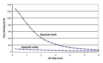
Reference Gear Magnetic Gradient Amplitude versus Air Gap
