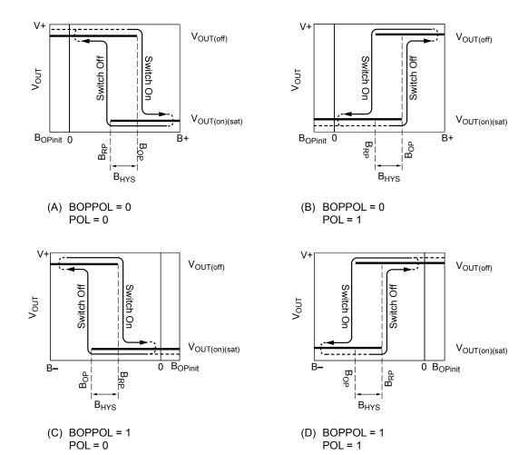
Figure 2. Hysteresis Diagrams. These plots demonstrate the behavior of the ATS128 with the applied magnetic field impinging on the branded face of the device case (refer to Package Outline Drawings section). On the horizontal axis, the B+ direction indicates increasing south or decreasing north magnetic flux density, and the B- direction indicates increasing north or decreasing south magnetic flux density.
