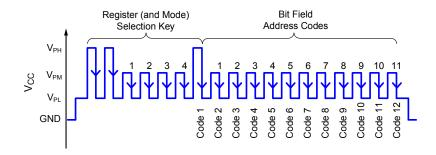
Figure 12. Example of Try mode programming pulses applied to the VCC pin. In this example,  $B_{OP}$  Positive Trim, Down-Counting register is addressed to code 12 by the eleven  $V_{PM}$  pulses (code 1 is selected automatically at the falling edge of the register-mode selection key).
