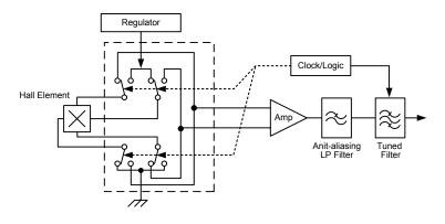
Figure 5. Concept of Chopper Stabilization Technique
