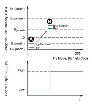
Figure 16. Positive Trim, Up-Counting to find  $B_{RP}$ .
