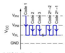
Figure 8. Try mode bit field addressing pulses.
