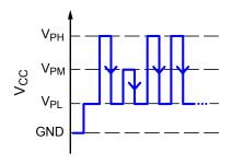
Figure 7. Example of Try mode register selection pulses, for the  $B_{\text{OP}}$  Negative Trim, Up-Counting register.
