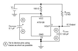
Figure 4. Typical Application Circuit
