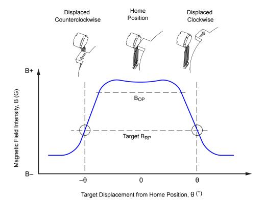
Figure 15. Example of magnetic flux density versus target displacement. In an application, an increasing B value could indicate either an increasing intensity of a south field or a decreasing intensity of a north field.
