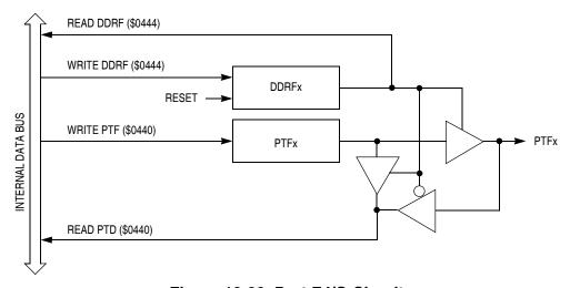
Figure 12-22. Port F I/O Circuit
