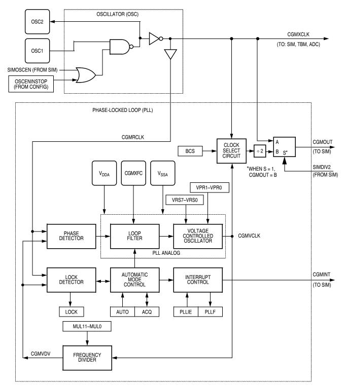
Figure 4-1. CGM Block Diagram
