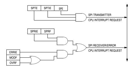
Figure 15-12. SPI Interrupt Request Generation
