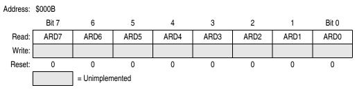
Figure 13-20. ESCI Arbiter Data Register (SCIADAT)
