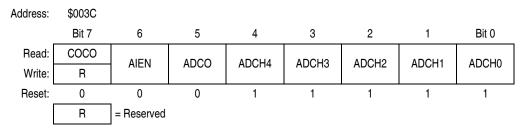
Figure 3-4. ADC Status and Control Register (ADSCR)
