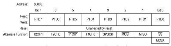
Figure 12-13. Port D Data Register (PTD)
