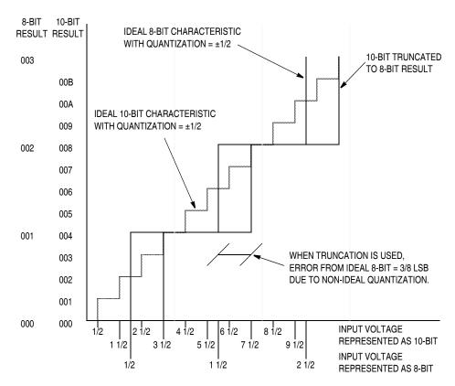
Figure 3-3. Bit Truncation Mode Error
