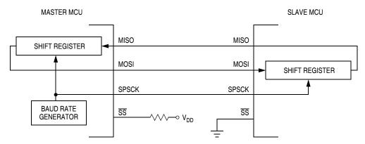
Figure 15-4. Full-Duplex Master-Slave Connections
