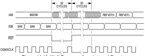
Figure 14-18. Wait Recovery from Internal Reset
