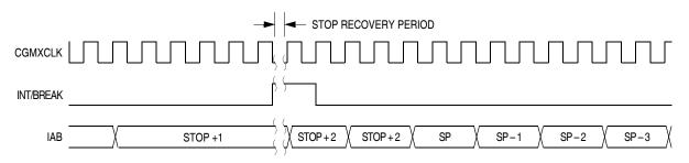
Figure 14-20. Stop Mode Recovery from Interrupt
