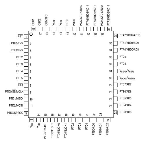
Figure 1-3. 48-Pin LQFP Pin Assignments
