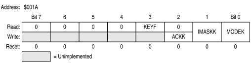
Figure 9-4. Keyboard Status and Control Register (INTKBSCR)
