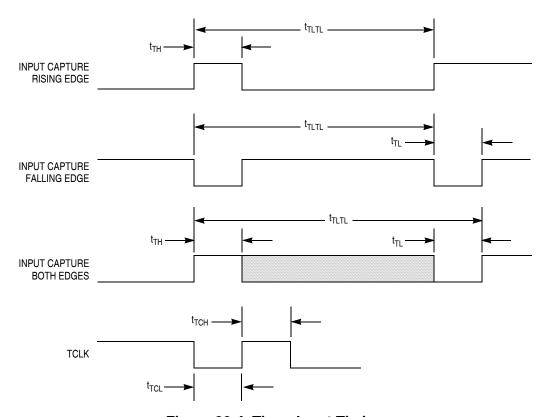
Figure 20-4. Timer Input Timing
