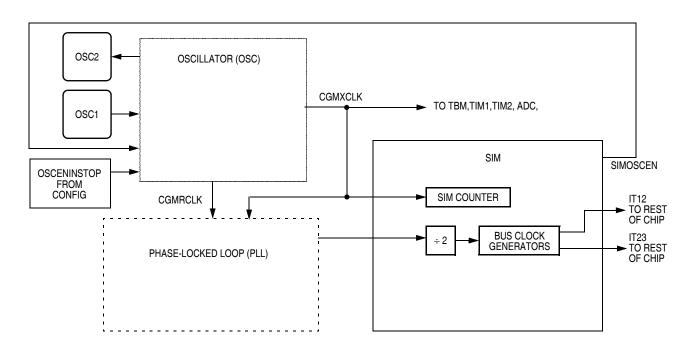
Figure 14-3. System Clock Signals
