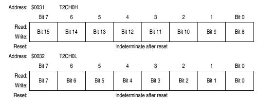
Figure 18-10. TIM2 Channel Registers (T2CH0H/L:T2CH5H/L) (Sheet 1 of 3)
