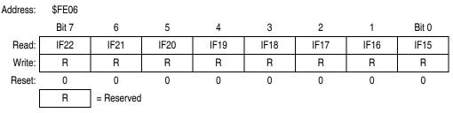
Figure 14-14. Interrupt Status Register 3 (INT3)
