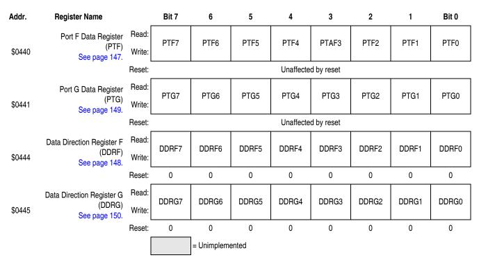
Figure 12-1. I/O Port Register Summary (Sheet 3 of 3)
