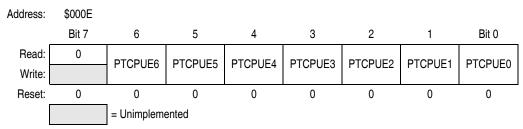
Figure 12-12. Port C Input Pullup Enable Register (PTCPUE)
