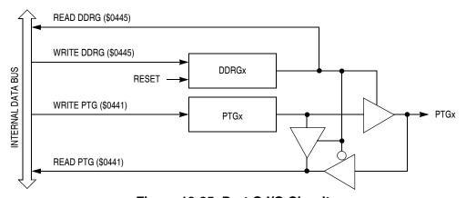
Figure 12-25. Port G I/O Circuit
