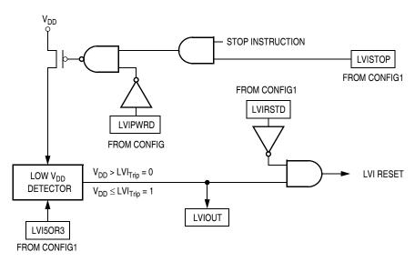
Figure 11-1. LVI Module Block Diagram
