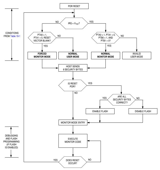
Figure 19-9. Simplified Monitor Mode Entry Flowchart
