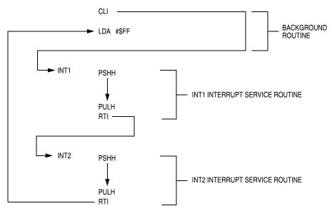
Figure 14-11. Interrupt Recognition Example
