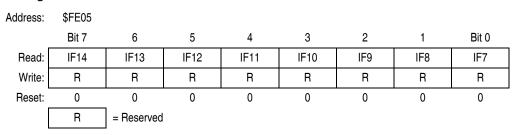
Figure 14-13. Interrupt Status Register 2 (INT2)
