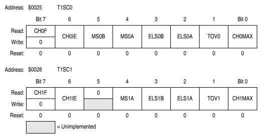
Figure 17-8. TIM1 Channel Status and Control Registers (T1SC0:T1SC1)
