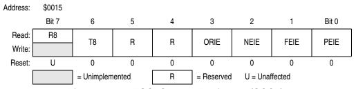
Figure 13-12. ESCI Control Register 3 (SCC3)
