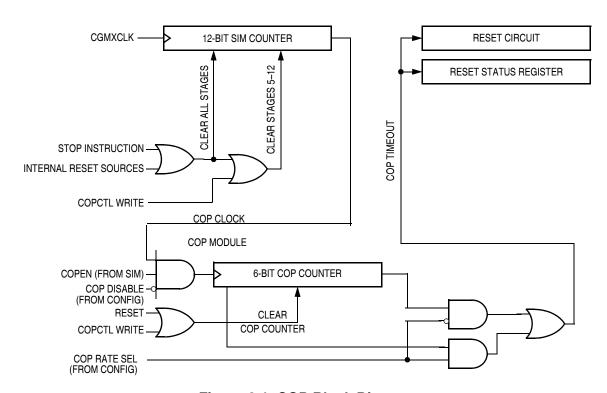
Figure 6-1. COP Block Diagram
