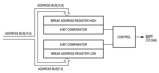
Figure 19-2. Break Module Block Diagram
