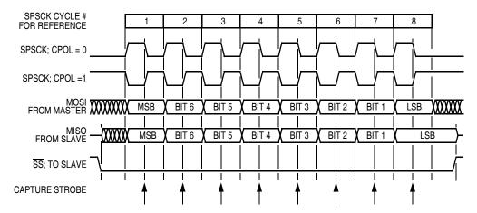
Figure 15-7. Transmission Format (CPHA = 1)
