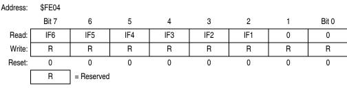
Figure 14-12. Interrupt Status Register 1 (INT1)
