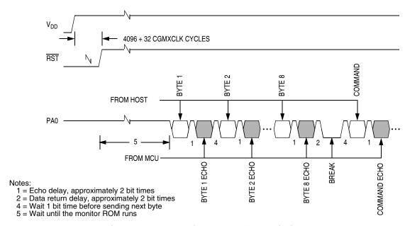
Figure 19-17. Monitor Mode Entry Timing
