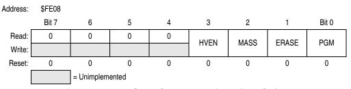
Figure 2-3. FLASH-1 Control Register (FL1CR)
