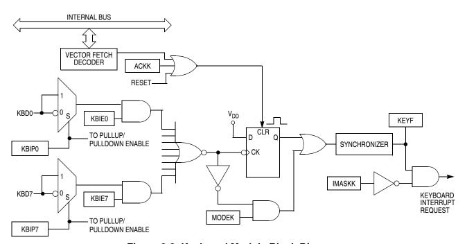
Figure 9-2. Keyboard Module Block Diagram
