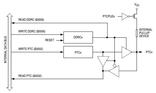
Figure 12-11. Port C I/O Circuit
