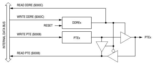
Figure 12-19. Port E I/O Circuit
