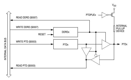
Figure 12-15. Port D I/O Circuit
