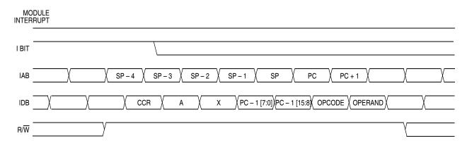
Figure 14-9. Interrupt Recovery Timing
