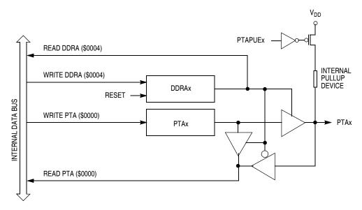
Figure 12-4. Port A I/O Circuit
