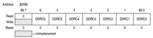
Figure 12-10. Data Direction Register C (DDRC)
