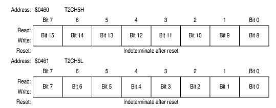
Figure 18-10. TIM2 Channel Registers (T2CH0H/L:T2CH5H/L) (Sheet 3 of 3)
