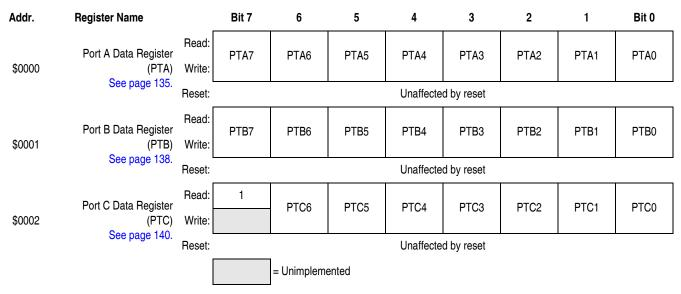
Figure 12-1. I/O Port Register Summary (Sheet 1 of 3)
