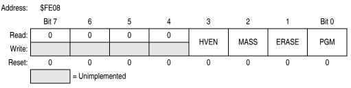
Figure 2-7. FLASH-2 Control Register (FL2CR)
