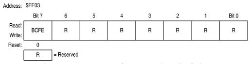
Figure 19-8. Break Flag Control Register (BFCR)
