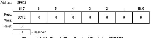
Figure 14-23. Break Flag Control Register (BFCR)
