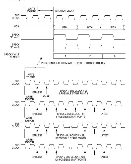
Figure 15-8. Transmission Start Delay (Master)
