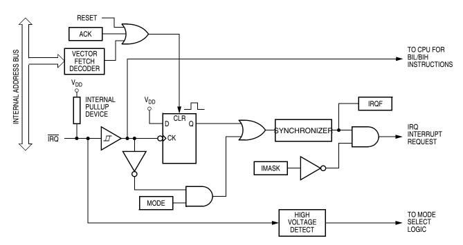
Figure 8-1. IRQ Module Block Diagram
