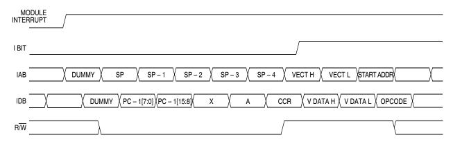
Figure 14-8. Interrupt Entry Timing
