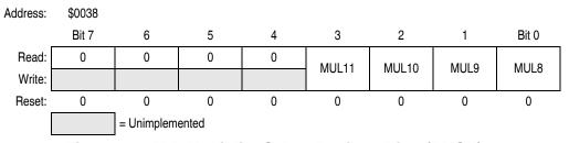
Figure 4-6. PLL Multiplier Select Register High (PMSH)
