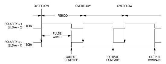
Figure 18-4. PWM Period and Pulse Width
