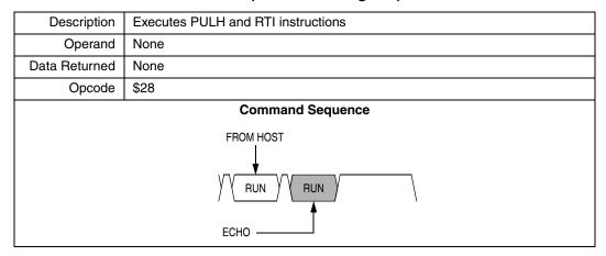
The MCU executes the SWI and PSHH instructions when it enters monitor mode. The RUN command tells the MCU to execute the PULH and RTI instructions. Before sending the RUN command, the host can modify the stacked CPU registers to prepare to run the host program. The READSP command returns the incremented stack pointer value, SP + 1. The high and low bytes of the program counter are at addresses SP + 5 and SP + 6.
