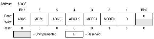
Figure 3-9. ADC Clock Register (ADCLK)
