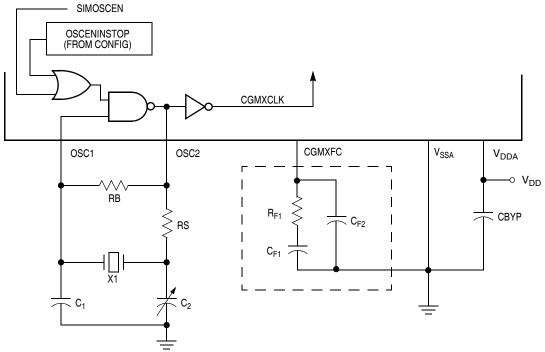
Note: Filter network in box can be replaced with a single capacitor, but will degrade stability.
