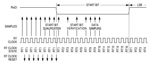
Figure 13-7. Receiver Data Sampling
