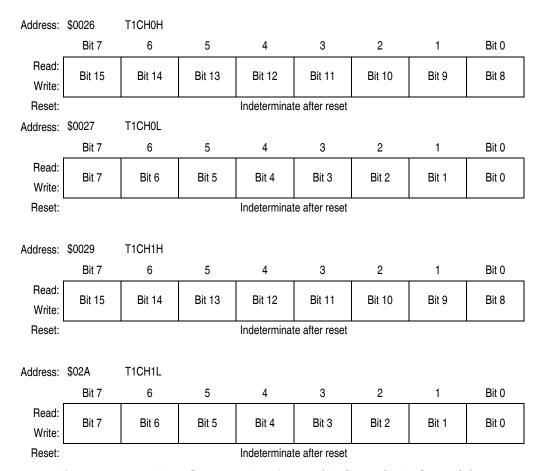
Figure 17-10. TIM1 Channel Registers (T1CH0H/L:T1CH1H/L)
