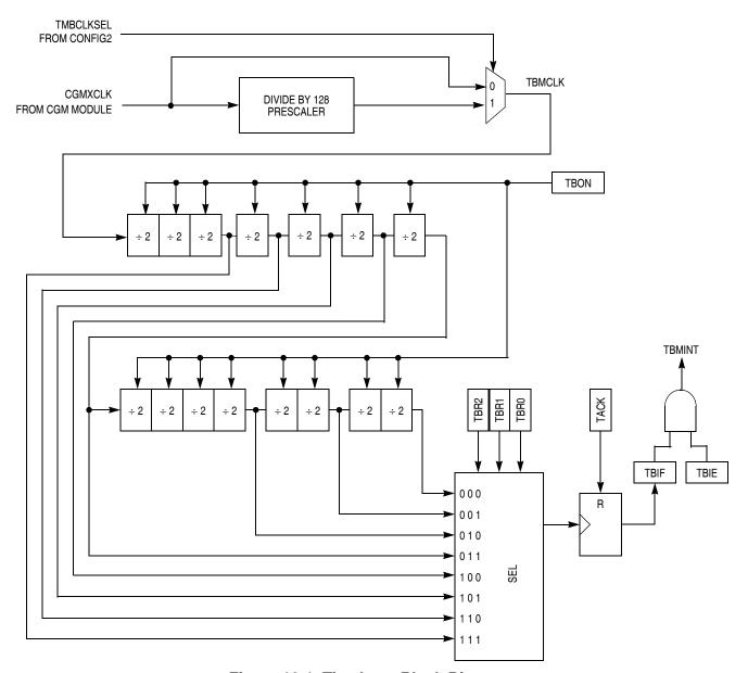
Figure 16-1. Timebase Block Diagram
