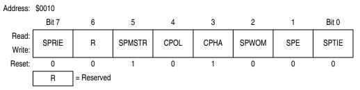
Figure 15-14. SPI Control Register (SPCR)
