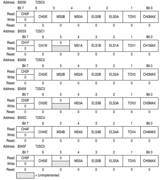
Figure 18-8. TIM2 Channel Status and Control Registers (T2SC0:T2SC5)
