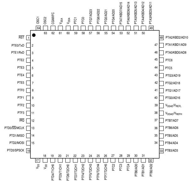
Figure 1-4. 64-Pin QFP Pin Assignments
