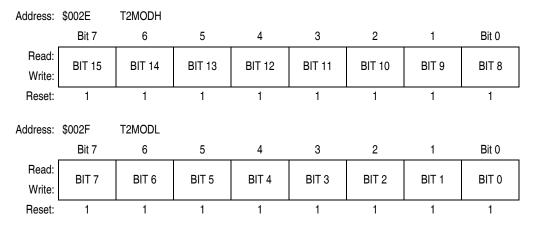
Figure 18-7. TIM2 Counter Modulo Registers (T2MODH and T2MODL)
