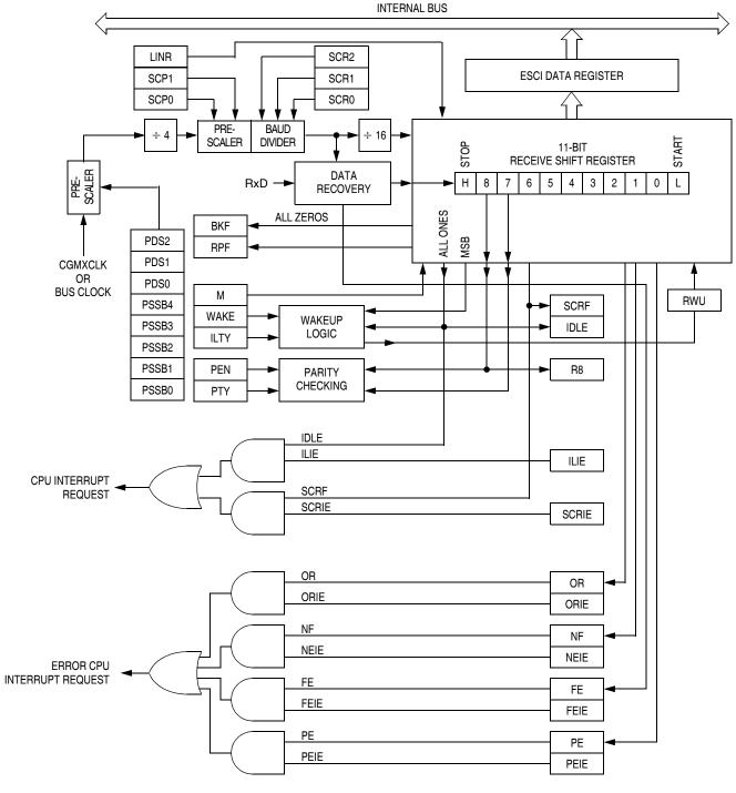
Figure 13-6. ESCI Receiver Block Diagram
