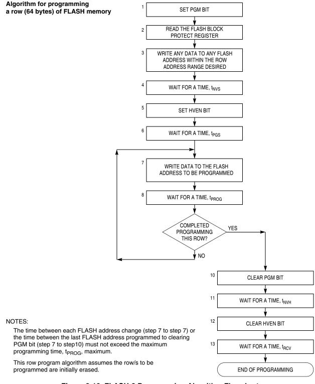
Figure 2-10. FLASH-2 Programming Algorithm Flowchart
