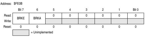
Figure 19-4. Break Status and Control Register (BRKSCR)
