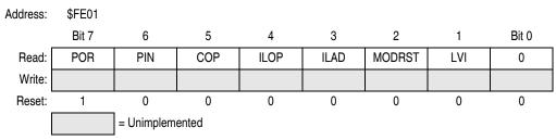
Figure 14-22. SIM Reset Status Register (SRSR)
