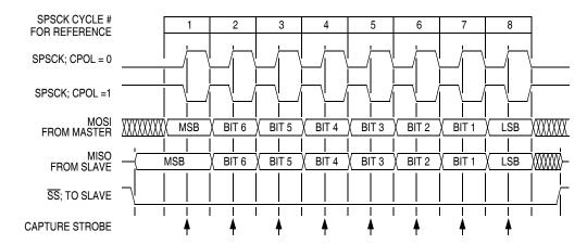
Figure 15-5. Transmission Format (CPHA = 0)
