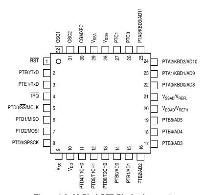
Figure 1-2. 32-Pin LQFP Pin Assignments
