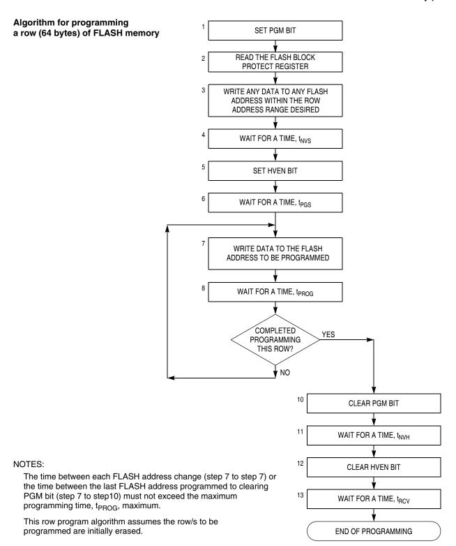
Figure 2-6. FLASH-1 Programming Algorithm Flowchart
