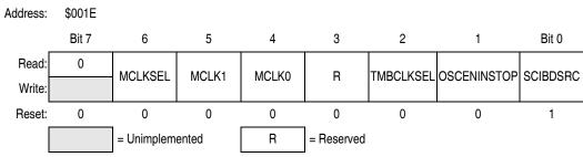
Figure 5-1. Configuration Register 2 (CONFIG2)
