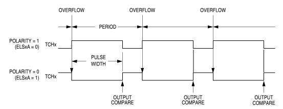
Figure 17-4. PWM Period and Pulse Width
