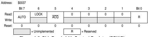
Figure 4-5. PLL Bandwidth Control Register (PBWC)
