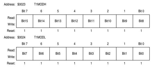
Figure 17-7. TIM1 Counter Modulo Registers (T1MODH:T1MODL)
