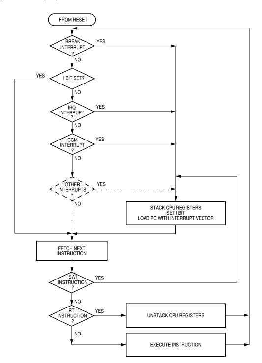
Figure 14-10. Interrupt Processing
