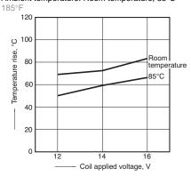
1-(2). Coil temperature rise (15A) Measured portion: Inside the coil Contact carrying current, 15A Ambient temperature: Room temperature, 85°C
