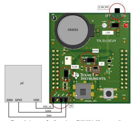
Figure 8. Jumpers Configuration – EVM With Microcontroller
