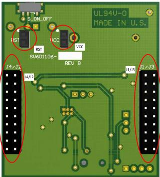
Figure 9. Jumpers Configuration – EVM With LaunchPad
