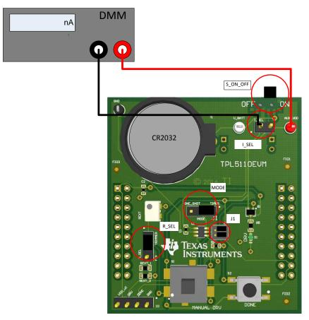
Figure 10. Current Measurement Setup - TPL5110 only
