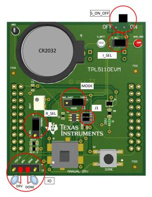
Figure 7. Jumpers Configuration – EVM Standalone Without Microcontroller
