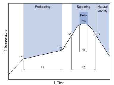
Preheating Soldering Peak Time Temp. Temp. Time Temp. Time T1 T2 **T**4 t1 ТЗ t2 t3 150°C 180°C 90 to 120s 230°C 40s 255°C 10s max.
